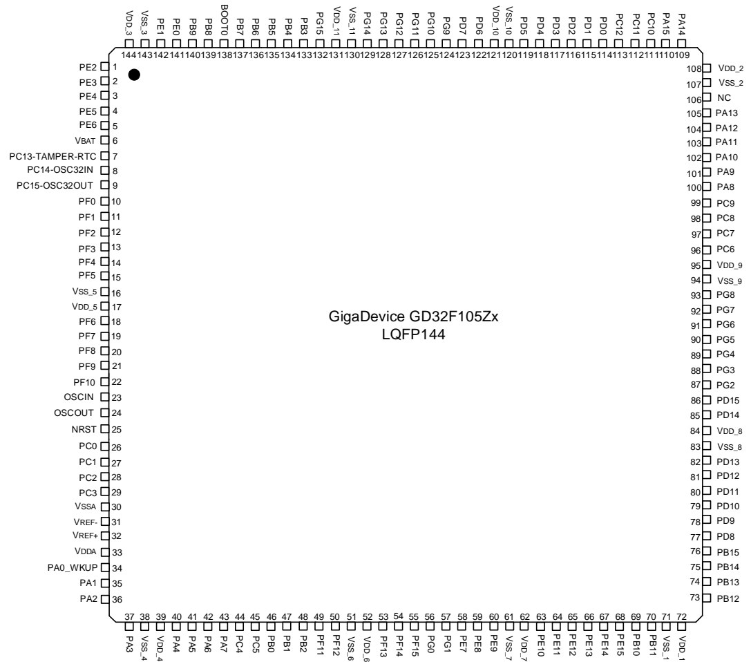
Figure 2-2. GD32F105Zx LQFP144 pinouts
