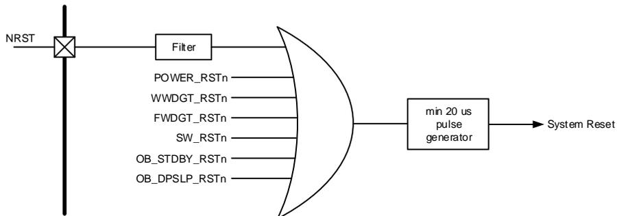
Figure 2-7. Recommend External Reset Circuit
