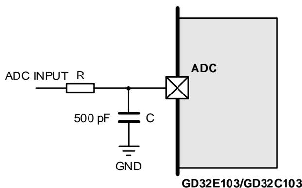
When  $f_{ADC} = 42\text{MHz}$ , the relationship between input impedance and sampling period is as follows. In order to obtain better conversion results, it is recommended to reduce the frequency of  $f_{ADC}$  as much as possible, and select a larger sampling period as much as possible. In the design of external circuit, input impedance should also be reduced as much as possible.
