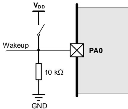
**Note:** This mode needs to be noted in circuit design, if there is a series resistance between PA0 and VDD, it may increase additional power consumption.
