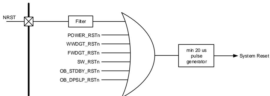
Figure 2-17. Recommend External Reset Circuit
