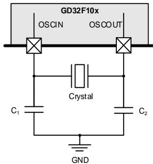
Figure 2-20. HXTAL External Clock Circuit
