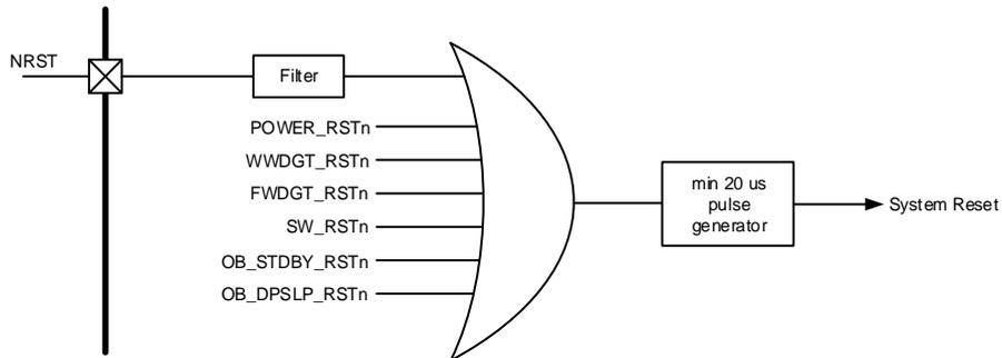
Figure 2-7. Recommend External Reset Circuit
