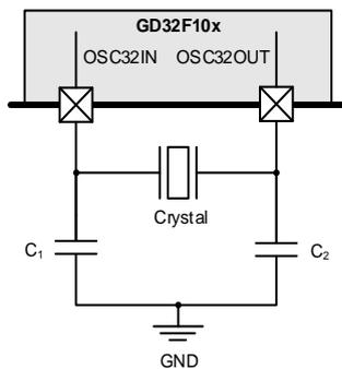
Figure 2-22. LXTAL External Clock Circuit
