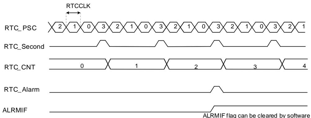
Figure 17-3. RTC second and overflow waveform example (RTC\_PSC= 3)
