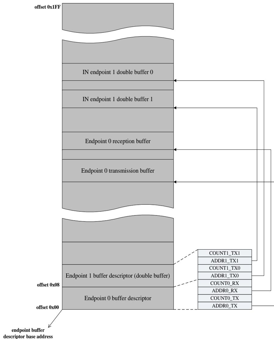
**Note:** This figure is not drawn on the actual scale, and it is addressed through the USB bus 16-bit mode.
