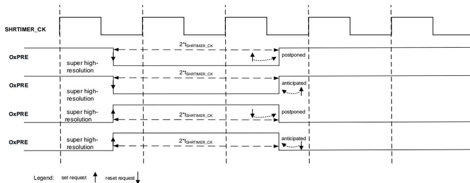
If the “set and reset requests” are generated with an interval including more than two complete  $t_{HPTMER\_CK}$  periods, the super high-resolution is available. Refer to [Figure 19-23. Super high-resolution OxpRE wave](#).
