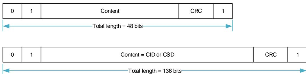
A response always starts with a start bit (always 0), followed by the bit indicating the direction of transmission (card = 0). A value 'x' in the tables below indicates a variable entry. All responses except for the type R3 are protected by a CRC. Every command code word is terminated by the end bit (always 1).
