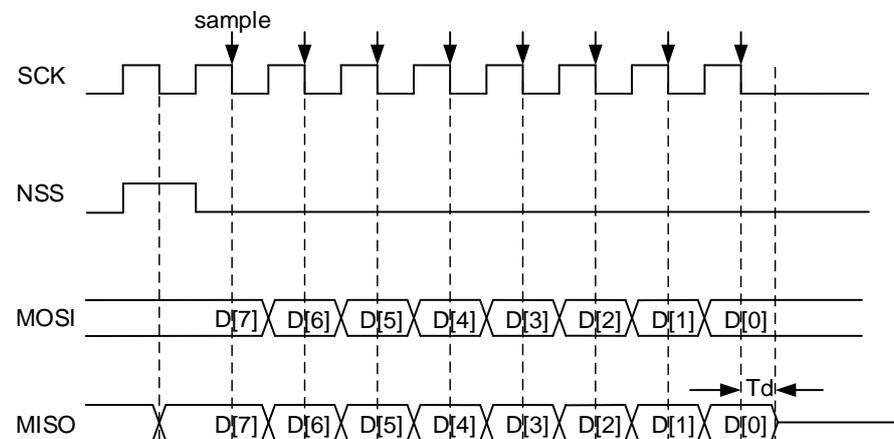
In slave TI mode, after the last rising edge of SCK in transfer, the slave begins to transmit the
