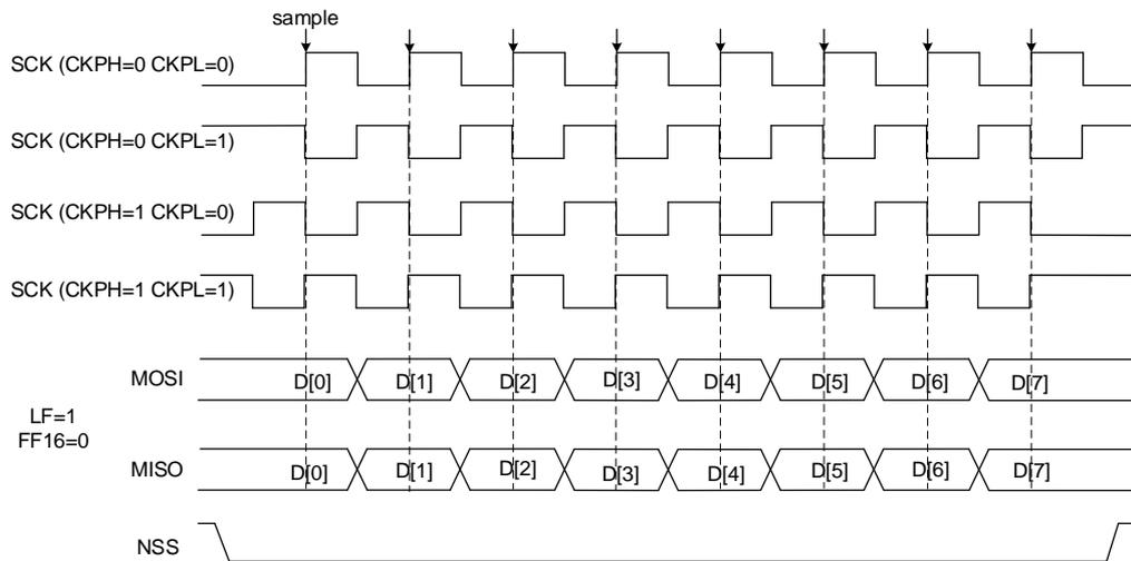
In SPI normal mode, the length of data is configured by the FF16 bit in the SPI\_CTL0 register. Data length is 16 bits if FF16=1, otherwise is 8 bits. Data order is configured by LF bit in SPI\_CTL0 register, and SPI will send the LSB first if LF=1, or the MSB if LF=0. The data order is fixed to MSB first in TI mode.
