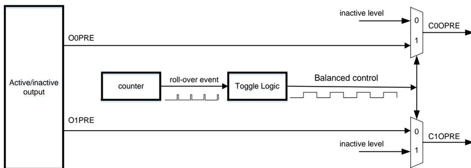
Once receiving roll-over event, the output of toggle logic module toggles. When the output of toggle logic module is 1 (high level), C0OPRE is connected to O0PRE and C1OPRE is set to
