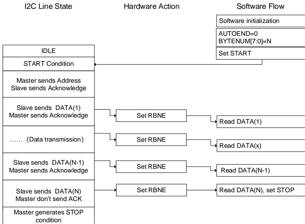
**Figure 21-34. Programming model for master receiving (N>255)**
