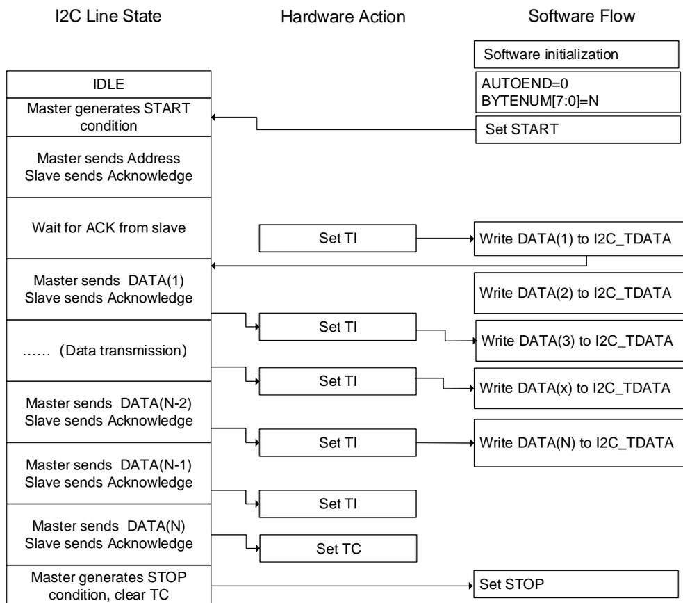
**Figure 21-32. Programming model for master transmitting (N>255)**
