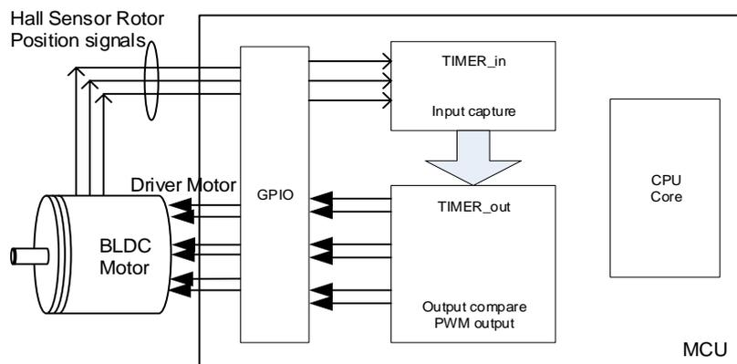
Figure 18-23. Hall sensor timing between two timers
