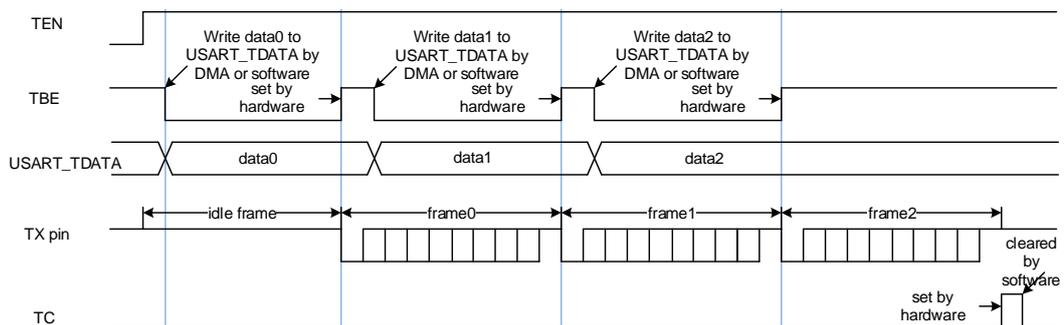
It is necessary to wait for the TC bit to be asserted before disabling the USART or entering the power saving mode. The TC bit can be cleared by writing 1 to TCC bit in USART\_INTC register.
