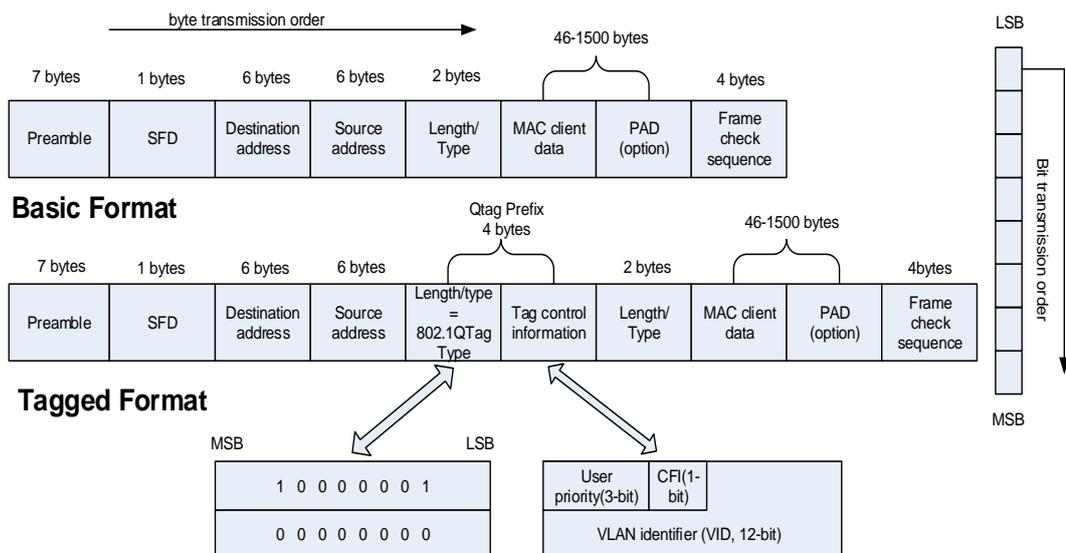
**Note:** The Ethernet controller transmits each byte at LSB first except FCS field.
