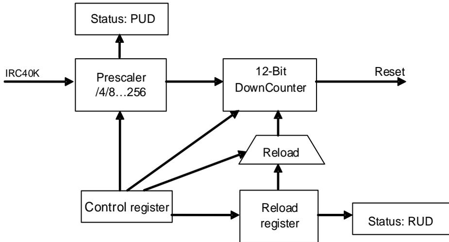
The free watchdog is enabled by writing the value (0xCCCC) to the control register (FWDGT\_CTL), then the counter starts counting down. When the counter reaches the value (0x000), there will be a reset.
