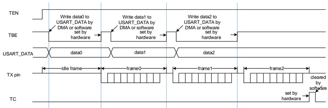
It is necessary to wait for the TC bit to be asserted before disabling the USART or entering the power saving mode. This bit can be cleared by a software sequence: reading the USART\_STAT0 register and then writing the USART\_DATA register. If the multibuffer communication is selected (DENT=1), this bit can also be cleared by writing 0 directly.
