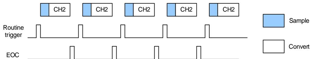
After conversion of a single routine channel, the conversion data will be stored in the ADC\_RDATA register, the EOC will be set. An interrupt will be generated if the EOCIE bit is set.
