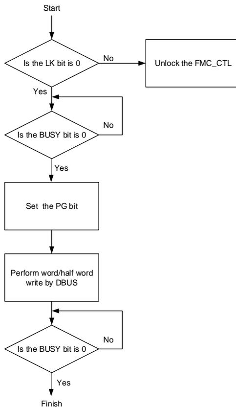
**Note:** Reading the flash should be avoided when a program/erase operation is ongoing in the same bank. And flash memory accesses will fail if the CPU enters the power saving modes.
