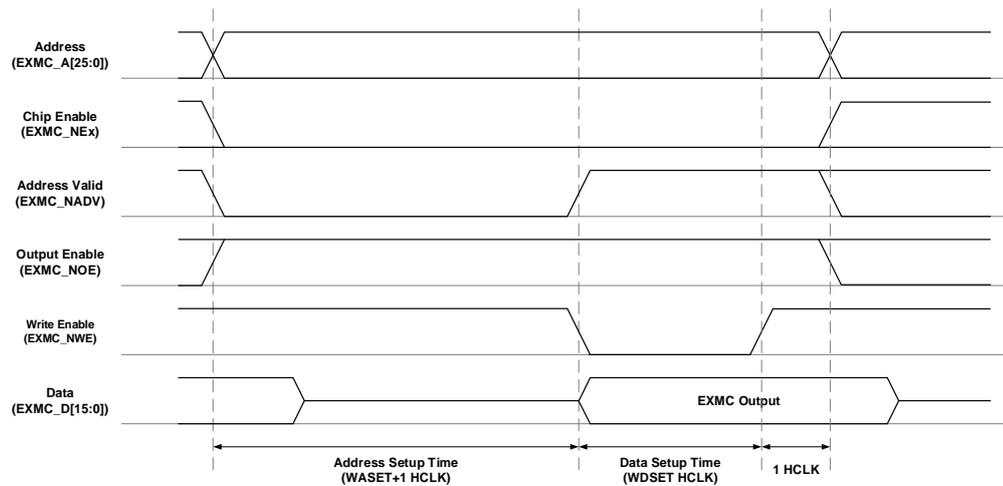
The differences between mode C and mode 1 write timing are that read/write timing is specified by the same set of timing configuration, while mode C write timing configuration is independent of its read configuration, and the toggle of NOE and NADV are different.
