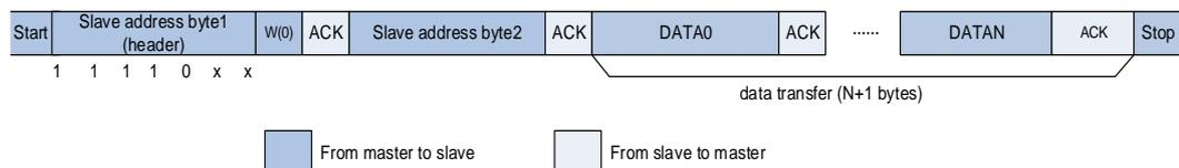
**Figure 21-18. I2C communication flow with 7-bit address (Master Transmit)**
