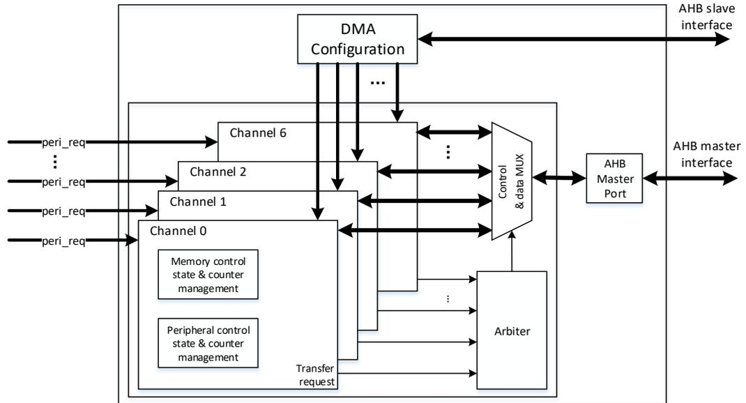
As shown in [Figure 11-1. Block diagram of DMA](#), a DMA controller consists of four main parts:
