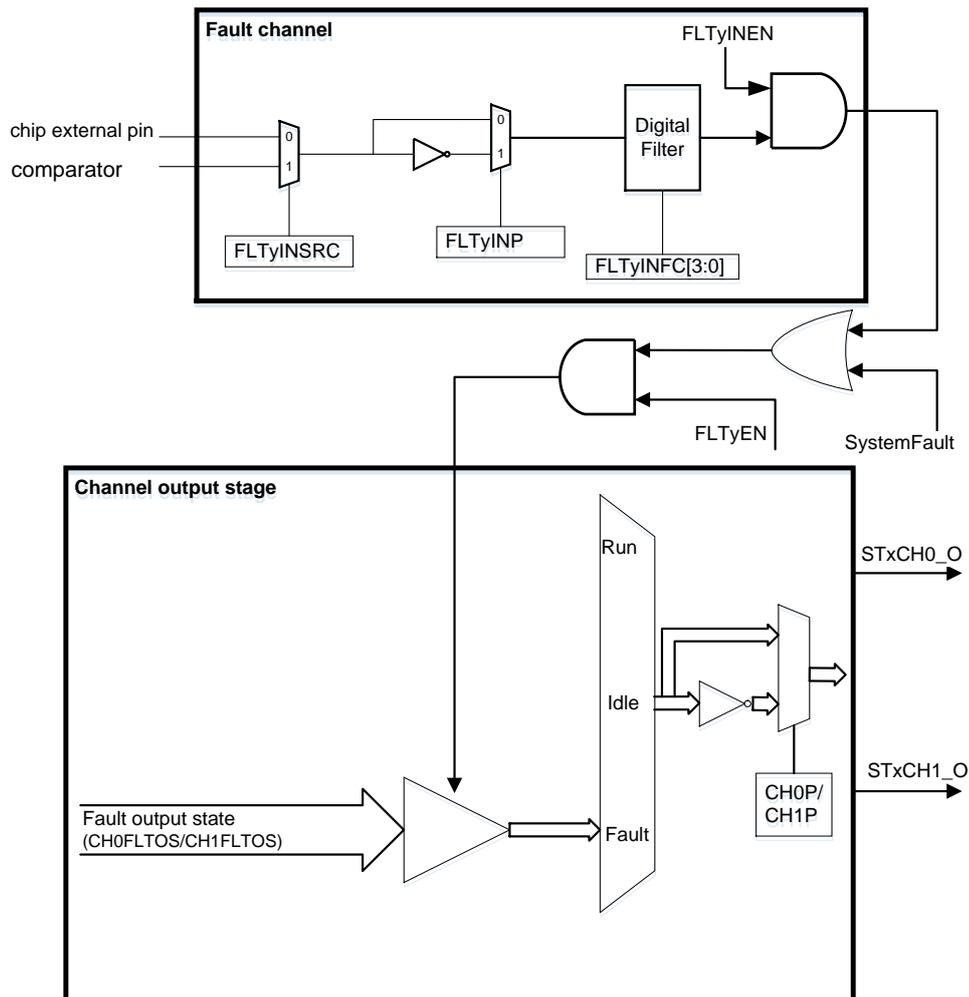
Fault input is enabled using FLTyEN bit in SHRTIMER\_STxFLTCTL register. A write-once FLTENPROT bit in the SHRTIMER\_STxFLTCTL register allows to protect FLTyEN bits for safety purpose. When FLTENPROT bit is set to 1, FLTyEN bits are writing protected (read-only).
