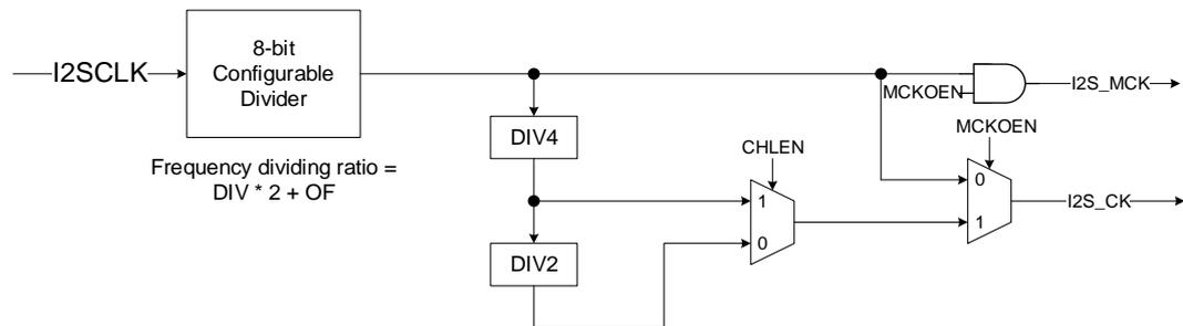
The block diagram of I2S clock generator is shown as [Figure 22-51. Block diagram of I2S clock generator](#). The I2S interface clocks are configured by the DIV bits, the OF bit, the MCKOEN bit in the SPI\_I2SPSC register and the CHLEN bit in the SPI\_I2SCTL register. The source clock is the system clock(CK\_SYS) or PLL2\*2. The I2S bitrate can be calculated by the formulas shown in [Table 22-7. I2S bitrate calculation formulas](#).
