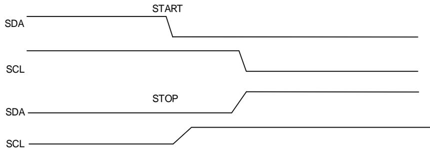
Each I2C device is recognized by a unique address (whether it is a microcontroller, LCD driver, memory or keyboard interface) and can operate as either a transmitter or receiver, depending on the function of the device. It operates in slave mode by default. When it generates a START signal, the interface automatically switches from slave to master. If an arbitration loss or a STOP generation occurs, then the interface switches from master to slave, allowing multimaster capability.
