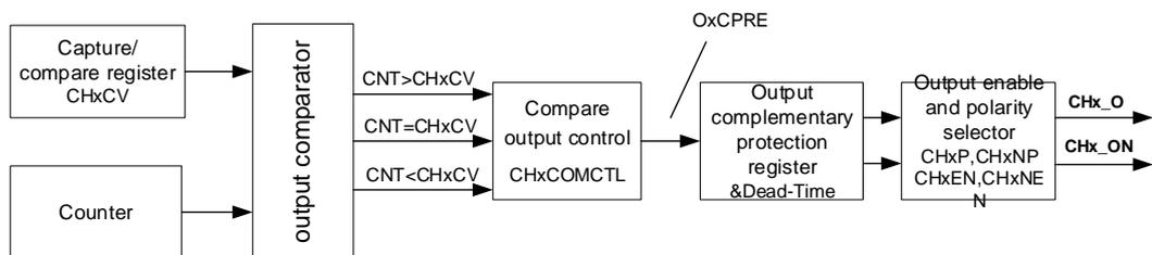
**Figure 18-14. Channel output compare principle (CH3\_O)**
