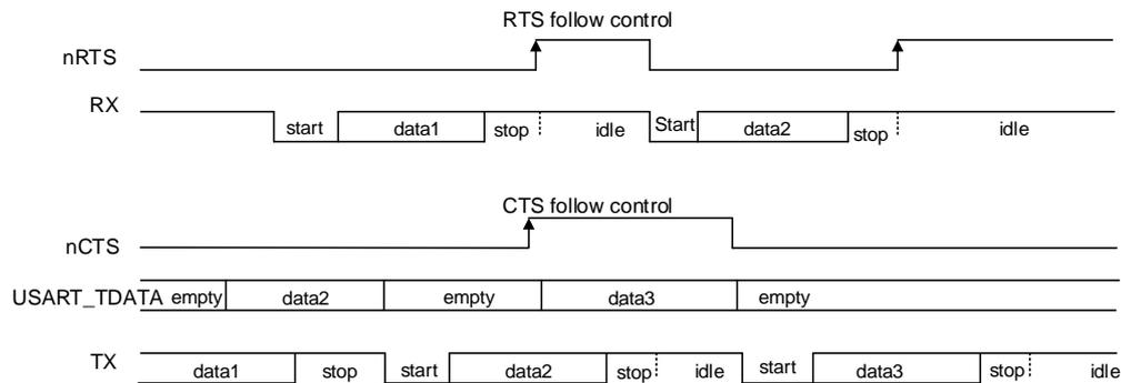
If the CTS flow control is enabled, the CTSF bit in USART\_STAT0 is set when the nCTS pin toggles. An interrupt is generated if the CTSIE bit in USART\_CTL2 is set.
