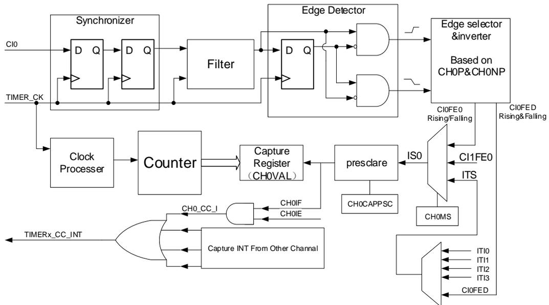
First, the channel input signal (`Cix`) is synchronized to `TIMER_CK` domain, and then sampled by a digital filter to generate a filtered input signal. Then through the edge detector, the rising and fall edge are detected. You can select one of them by `CHxP`. One more selector is for the other channel and trig, controlled by `CHxMS`. The `IC_prescaler` make several the input event generate one effective capture event. On the capture event, `TIMERx_CHxCV` will restore the value of counter.
