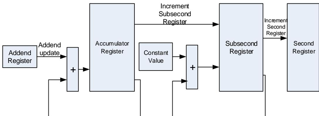
The following concrete example is used to describe the fine correction method how to update the system time:
