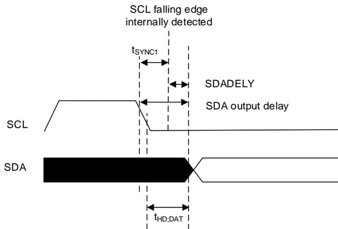
The SCLDELY counter starts when the data is sent on SDA output. As is shown in [Figure 21-23. Data setup time](#).
