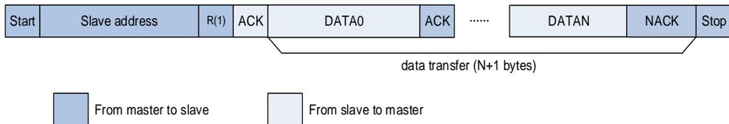
In 10-bit addressing mode, the HEAD10R bit can be configured to decide whether the complete address sequence must be executed, or only the header to be sent. When HEAD10R=0, the complete 10 bit address read sequence must be executed with START + header of 10-bit address in write direction + slave address byte 2 + RESTART + header of 10-bit address in read direction, as is shown in [Figure 21-20. I2C communication flow with 10-bit address \(Master Receive when HEAD10R=0\)](#).
