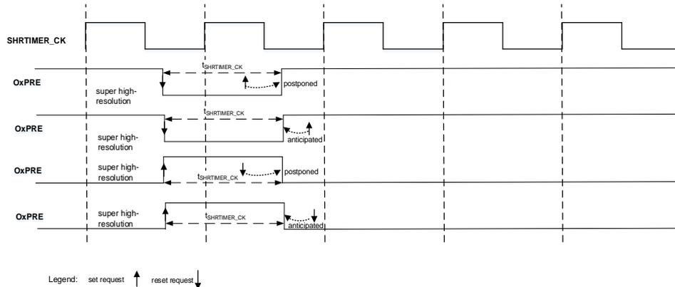
If the “set and reset requests” are generated with an interval including one complete  $t_{HPTMER\_CK}$  period, a pulse of 2  $t_{HPTMER\_CK}$  periods is generated. Refer to [Figure 19-22. A pulse of 2  \$t\_{SHRTMER\\_CK}\$  period](#).
