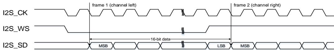
When the packet type is 16-bit data packed in 16-bit frame, only one write or read operation to or from the SPI\_DATA register is needed to complete the transmission of a frame.
