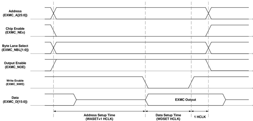
The difference between mode A and mode 1 write timing is that read/write timing is specified by the same set of timing configuration, while mode A write timing configuration is independent of its read configuration.
