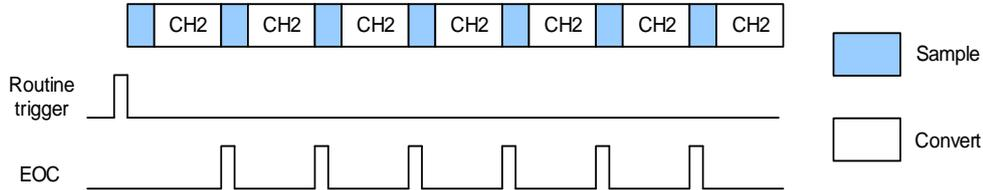
Software procedure for continuous conversion on a routine channel:
