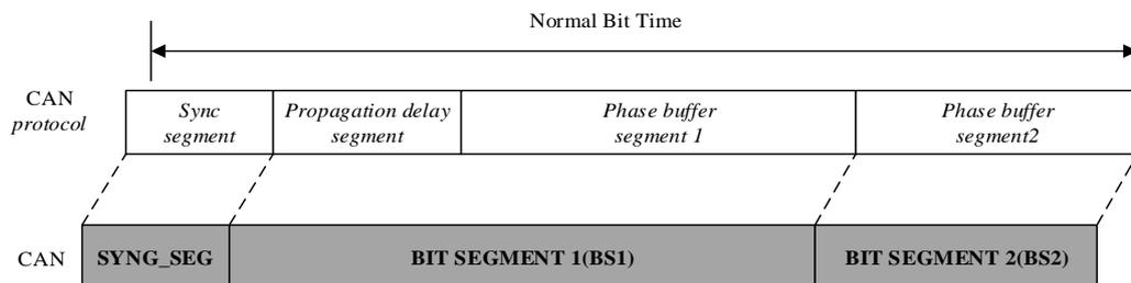
The resynchronization Jump Width (SJW): it can be lengthened or shortened to compensate for the Synchronization error of the CAN network node. It is programmable from 1 to 4 time quanta.
