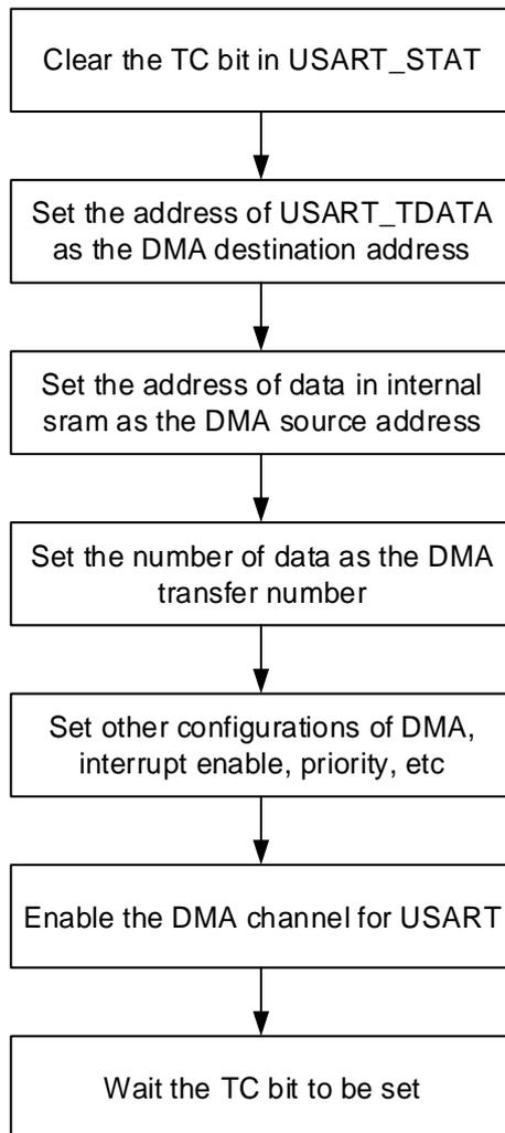
After all of the data frames are transmitted, the TC bit in USART\_STAT is set. An interrupt occurs if the TCIE bit in USART\_CTL0 is set.
