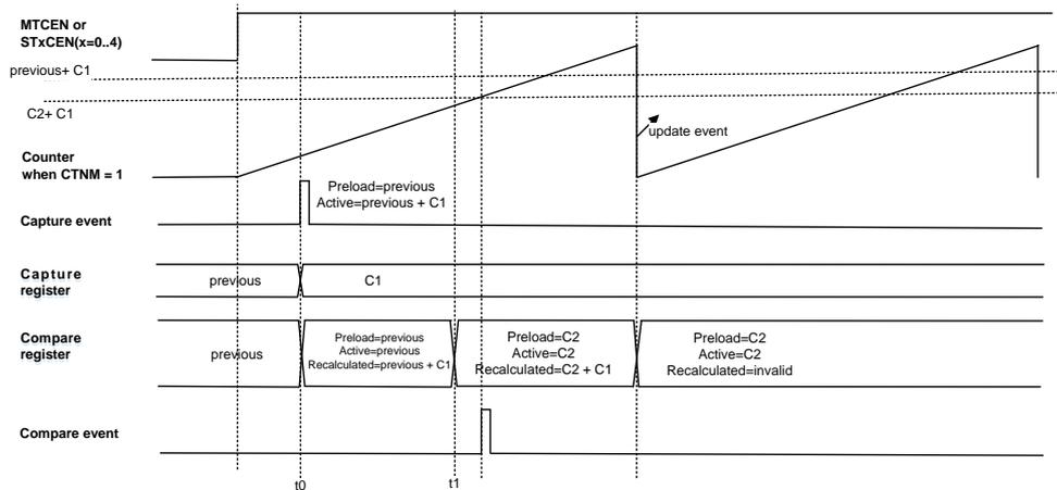
When the delayed mode is enabled (DELCMPyM[1:0]=01/10/11,y=1,3), the over-capture is prevented. In the same counting cycle (determined by SHRTIMER\_STxCAR), only the first capture event is taken into account. New capture event are effective in three cases as follows:
