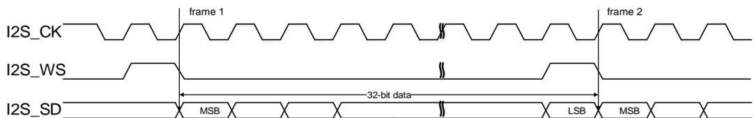
**Figure 22-39. PCM standard short frame synchronization mode timing diagram**
