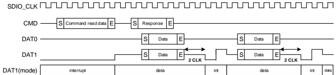
**Figure 24-18. Multiple block 4-Bit write interrupt cycle timing**
