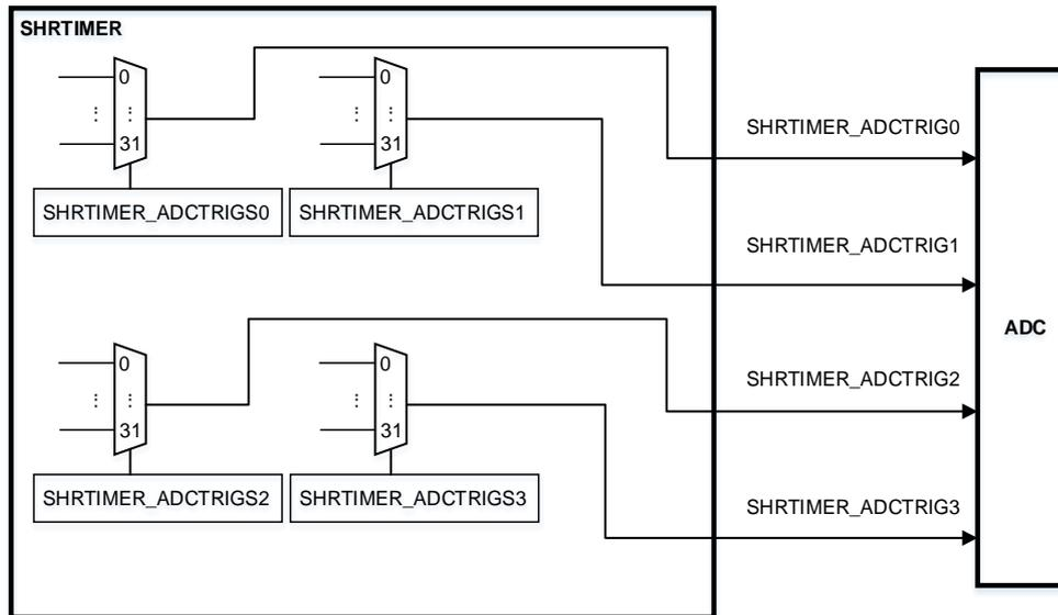
There are up to 32 events which can be combined (ORed) for each trigger output. They are defined in SHRTIMER\_ADCTRIGS<sub>y</sub>(y=0..3) registers.
