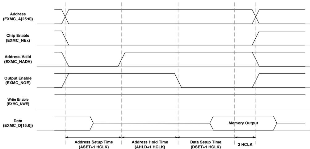
Figure 25-16. Mode D write access
