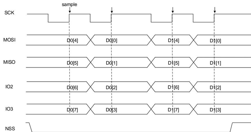
The data frame length is fixed to 8 bits in Quad-SPI mode.
