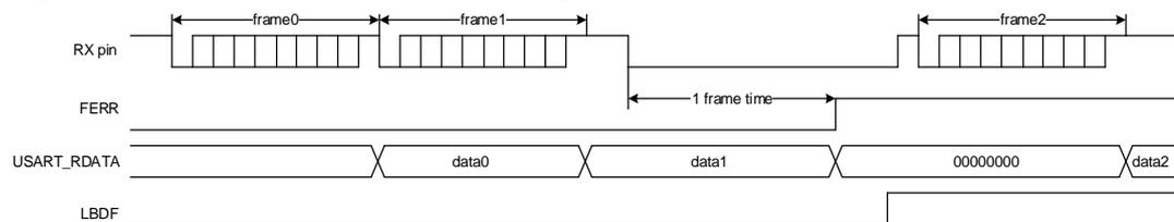
As shown in [Figure 20-24. Break frame occurs during a frame](#), if a break frame occurs during a frame on the RX pin, the FERR status will be asserted for the current frame.
