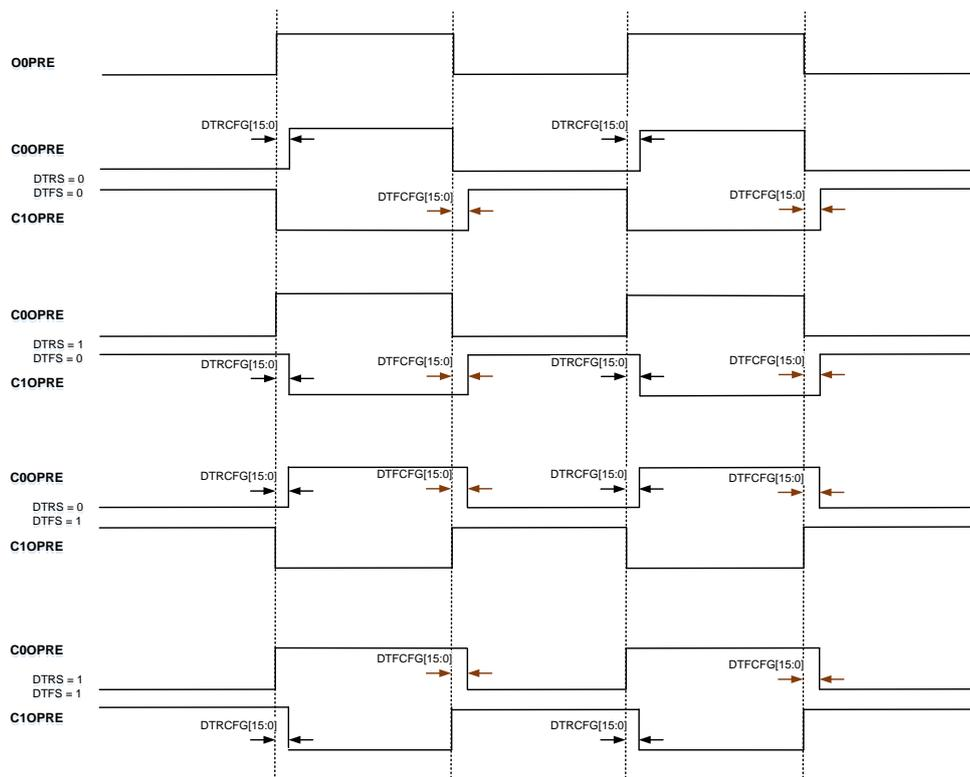
[Figure 19-27. Complementary wave with pulse width less than dead-time](#) shows C0OPRE and C1OPRE wave with O0PRE pulse width less than the dead-time.
