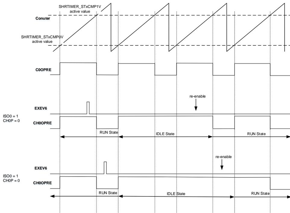
Figure 19-32. ISO0 = 0 and CHOP = 1 in delayed IDLE
