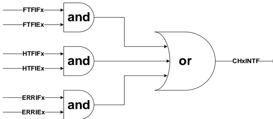
**NOTE:** “x” indicates channel number (for DMA0, x=0...6. for DMA1, x=0...4).
