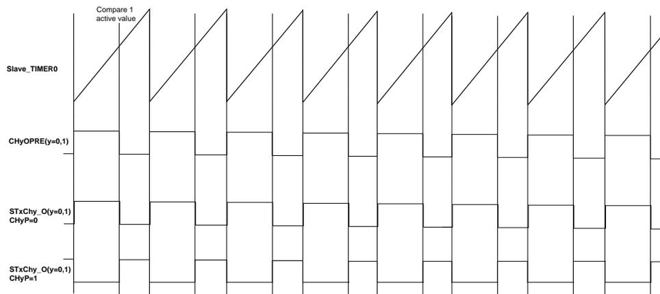
The output level in the Fault state is configured using CHyFLTOS[1:0] bits in SHRTIMER\_STxCHOCTL register, for each output, as follows:
