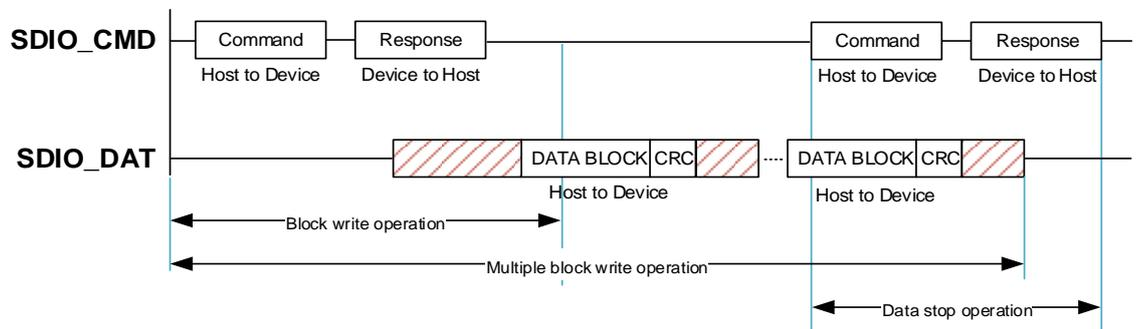
Data transfers to/from SD memory cards, SD I/O cards (both IO only card and combo card) and CE-ATA device are done in data blocks. Data transfers to/from MMC are done in data blocks or streams. [Figure 24-4. SDIO sequential read operation](#) and [Figure 24-5. SDIO sequential write operation](#) are the stream read and write operation.
