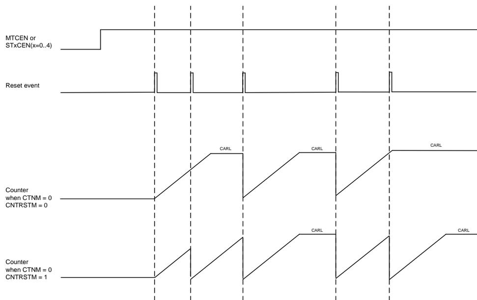
In continuous mode, the counter starts immediately as soon as MTCEN bit in SHRTIMER\_MTCTL0 register is set to 1. When counting up to the counter-reload value, the counter restarts from 0 and a roll-over event is generated. Different from single pulse mode, the reset events generated at any time will reset and restart the counter. [Figure 19-5. Counter behavior in continuous mode](#) shows counter operation diagram in continuous mode.
