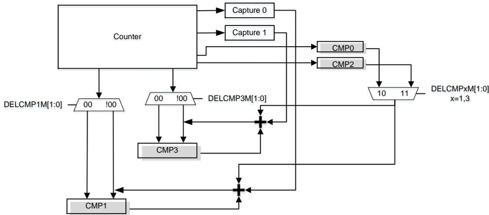
In delay mode, the compare y(y=1, 3) event is valid from the relative capture/compare event up to the period event. When the counter has reached the period value, the compare y(y=1, 3) event is disabled until a new capture/compare comes.
