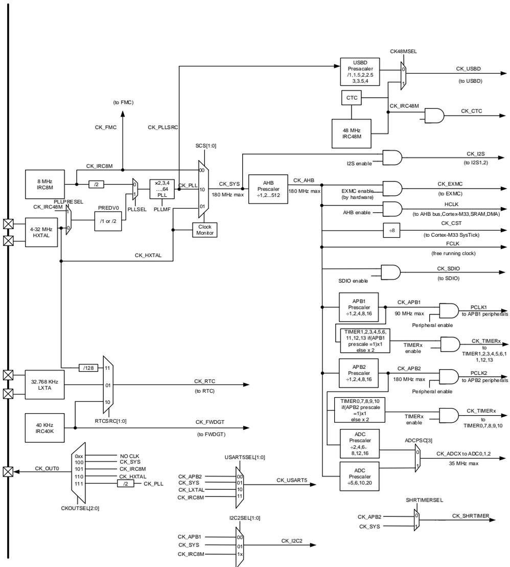
The frequency of AHB, APB2 and the APB1 domains can be configured by each prescaler. The maximum frequency of the AHB, APB2 and APB1 domains is 180 MHz / 180 MHz / 90 MHz. The Cortex® System Timer (SysTick) external clock is clocked with the AHB clock (HCLK) divided by 8. The SysTick can work either with this clock or with the AHB clock (HCLK), configurable in the systick control and status register.
