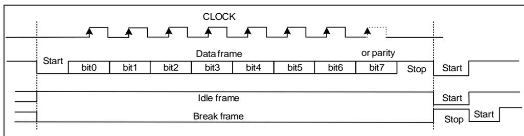
In transmission and reception, the number of stop bits can be configured by the STB[1:0] bits in the USART\_CTL1 register.
