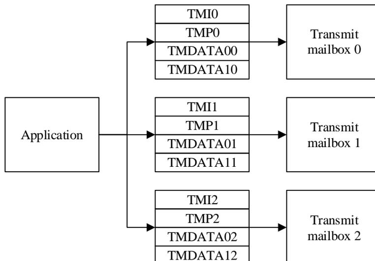
If FD frame would be transmitted, always write TMDATA00 registers when mailbox 0 is used, TMDATA01 register when mailbox 1 is used and TMDATA02 register when mailbox 2 is used until the end. For example, if application wants to transmit 64 bytes data using mailbox0, it needs to write the 64 bytes data through TMDATA00 register for 16 times. The data is stored in internal SRAM.
