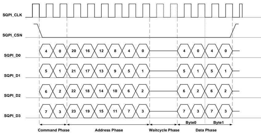
Figure 23-9. SQPI SSD Mode Timing
