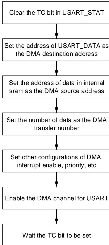
After all of the data frames are transmitted, the TC bit in USART\_STAT0 is set. An interrupt occurs if the TCIE bit in USART\_CTL0 is set.
