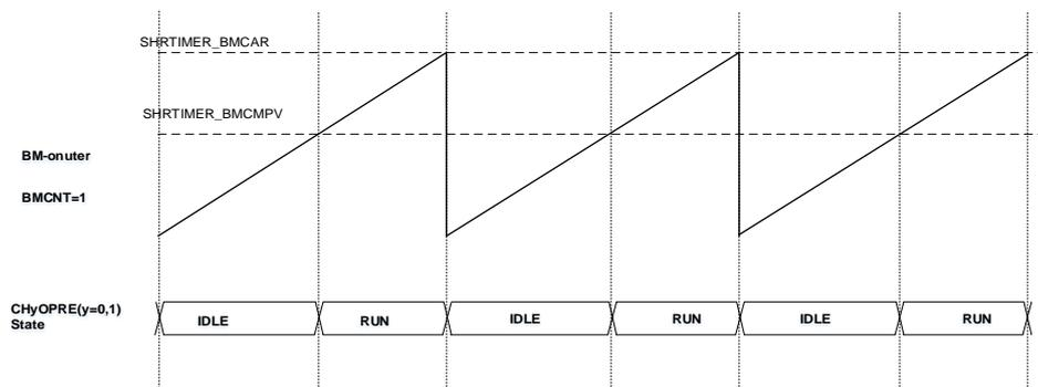
When BMSE is set, the SHRTIMER\_BMCMV and SHRTIMER\_BMCAR registers are preloaded and the transfer from preload to active register happens:
