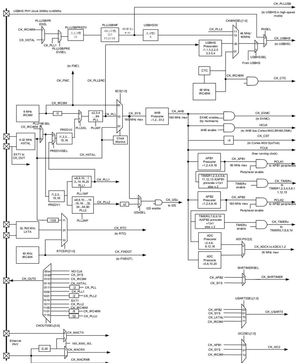
The frequency of AHB, APB2 and the APB1 domains can be configured by each prescaler. The maximum frequency of the AHB, APB2 and APB1 domains is 180 MHz / 180 MHz / 90 MHz. The Cortex® System Timer (SysTick) external clock is clocked with the AHB clock (HCLK) divided by 8. The SysTick can work either with this clock or with the AHB clock (HCLK), configurable in the systick control and status register.
