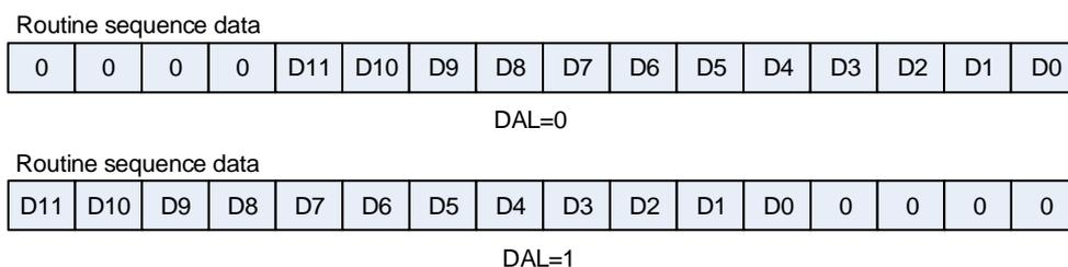
6-bit resolution data alignment is different from 12-bit/10-bit/8-bit resolution data alignment, shown as [Figure 13-9. 6-bit data storage mode](#)
