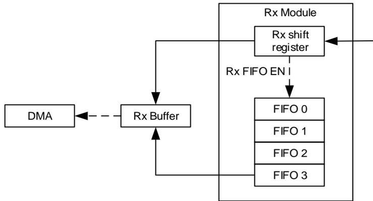
If the software read receive data buffer in the routing of the RBNE interrupt, the RBNEIE bit should be reset at the beginning of the routing and set after all of the receive data is read out. The PERR/NERR/FERR/EBF flags should be cleared before reading a receive data out.
