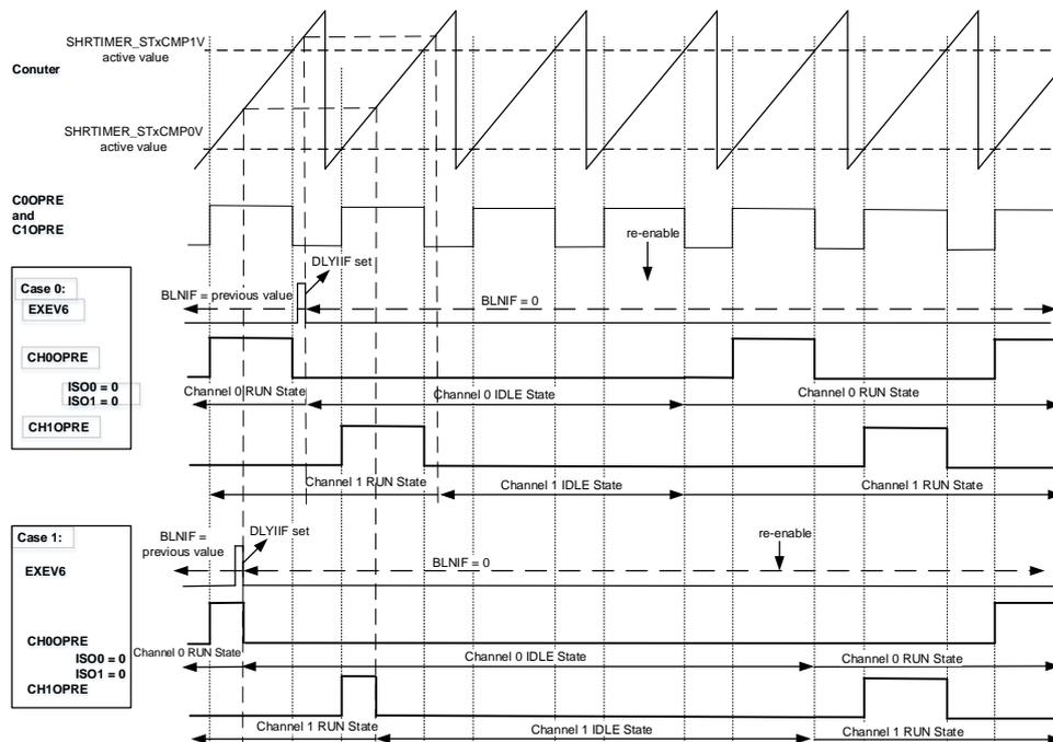
This BLNIF in SHRTIMER\_STxINTF register indicates which channel is outputting the signal when a balanced IDLE event entry occurred. For [Figure 19-34. Balanced IDEL with ISO0 = 0 and ISO1 = 0](#), external event 6 (EXEV6) arrives while channel 0 outputs the signal and channel 1 output inactive and BLNIF bit is reset to 0.
