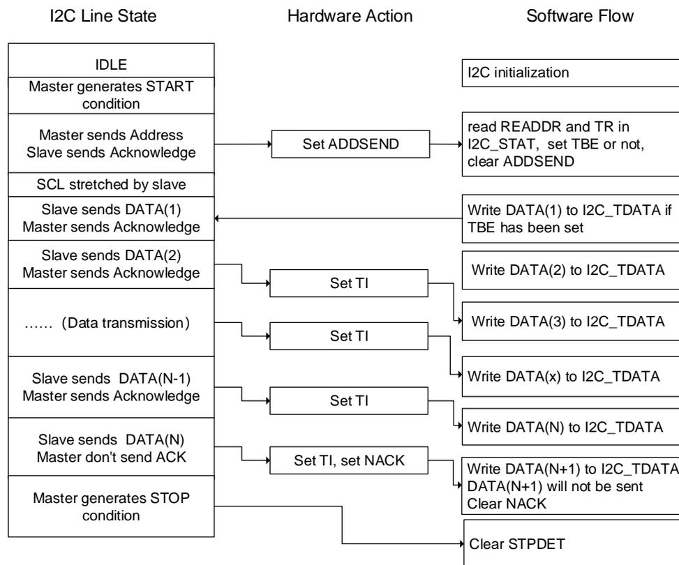
Figure 21-28. Programming model for slave transmitting when SS=1
