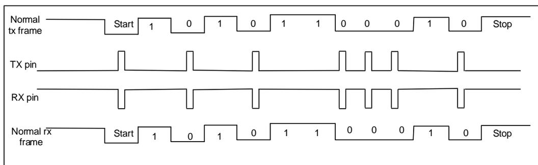
The SIR sub module can work in low power mode by setting the IRLP bit in USART\_CTL2. The transmit encoder is driven by a low speed clock, which is divided from the PCLK. The
