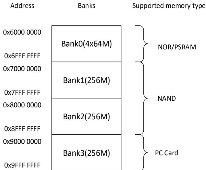
EXMC access space is divided into multiple banks. Each bank is 256 Mbytes. The first bank (Bank0) is further divided into four regions, and each region is 64 Mbytes. Bank $x$ ( $x=1, 2$ ) is divided into two spaces, the attribute memory space and the common memory space. Bank3 is divided into three spaces, which are the attribute memory space, the common memory space and the I/O memory space.
