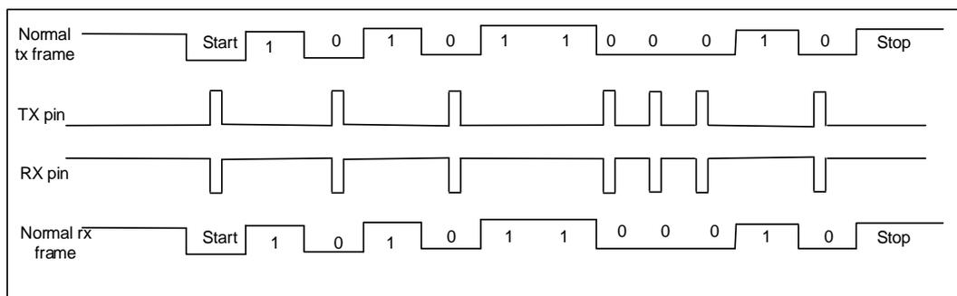
The SIR sub module can work in low power mode by setting the IRLP bit in USART\_CTL2. The transmit encoder is driven by a low speed clock, which is divided from the PCLK. The division ratio is configured by the PSC[7:0] bits in USART\_GP register. The pulse width on the TX pin is 3 cycles of this low speed period. The receiver decoder works in the same manner as the normal IrDA mode.
