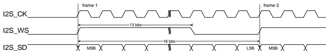
**Figure22-44. PCM standard long frame synchronization mode timing diagram**
