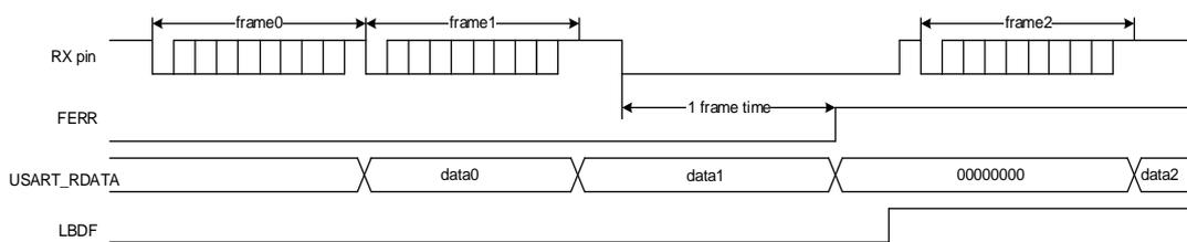
As shown in [Figure 20-10. Break frame occurs during a frame](#), if a break frame occurs during a frame on the RX pin, the FERR status will be asserted for the current frame.
