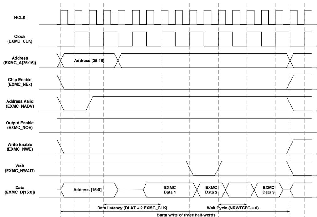
**Table 25-13. Timing configurations of synchronous multiplexed write mode**
