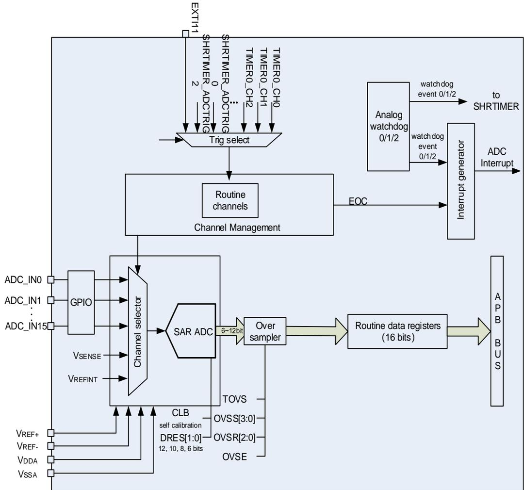
Figure 13-2. ADC module block diagram (for ADC2)
