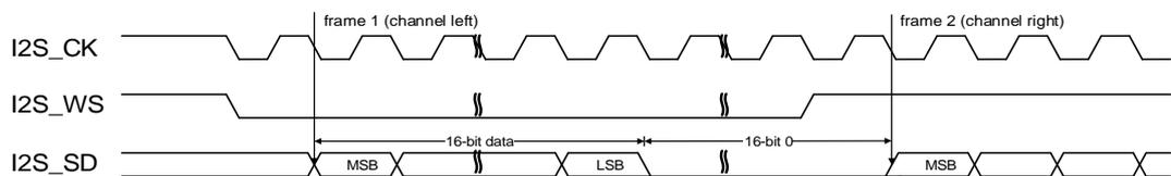
When the packet type is 16-bit data packed in 32-bit frame, only one write or read operation to or from the SPI\_DATA register is needed to complete the transmission of a frame. The remaining 16 bits are forced by hardware to 0x0000 to extend the data to 32-bit format.
