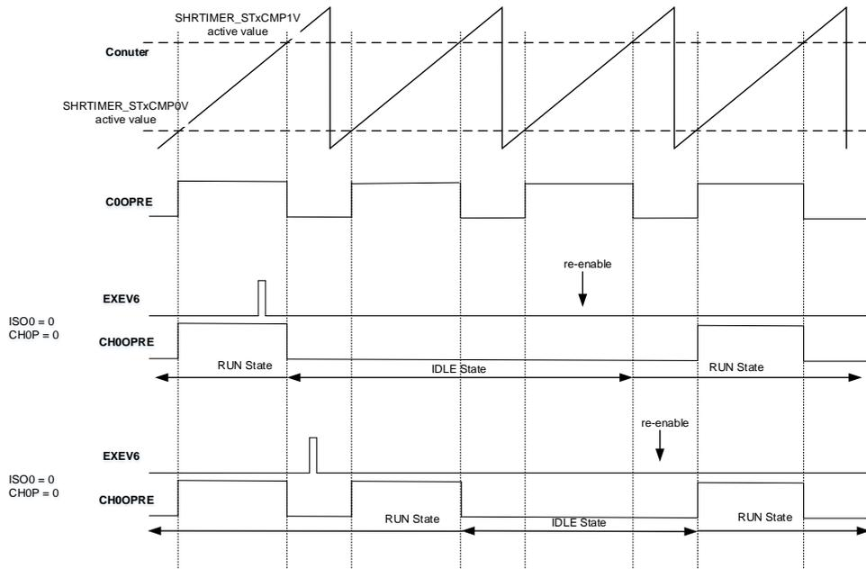
Figure 19-31. ISO0 = 1 and CHOP = 0 in delayed IDLE
