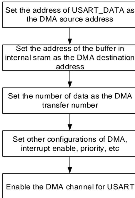
When the number of the data received by USART reaches the DMA transfer number, an end of transfer interrupt will be generated in the DMA module.
