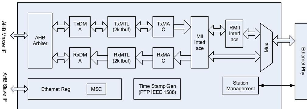
The MAC module is connected to the external PHY by MII or RMI through bit ENET\_PHY\_SEL in AFIO\_PCF0 register. The SMI (Station Management Interface) is used to configure and manage external PHY.
