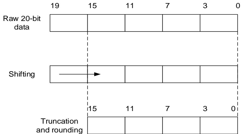
**Note:** If the intermediate result after the shifting exceeds 16 bits, the upper bits of the result are simply truncated.
