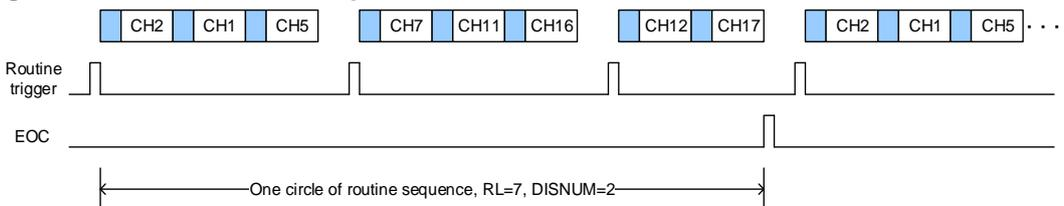
Software procedure for discontinuous conversion on a routine sequence:
