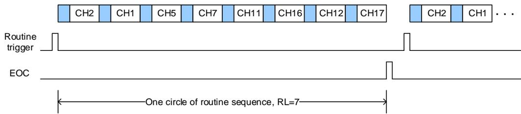
Software procedure for scan conversion on a routine sequence:
