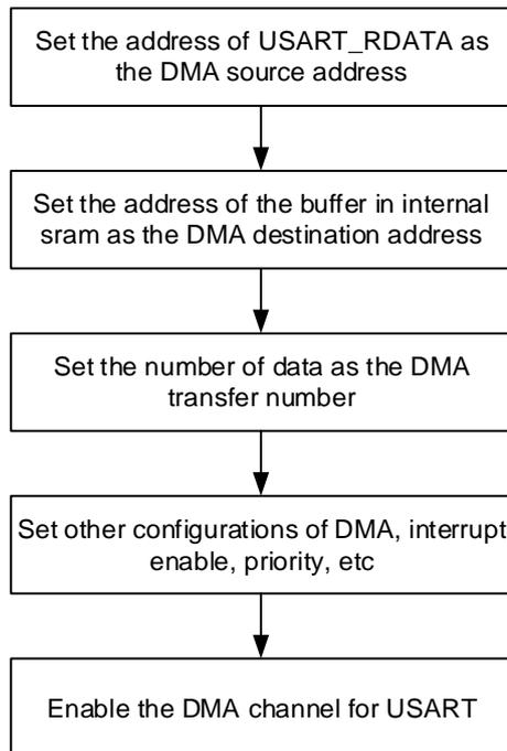
When the number of the data received by USART reaches the DMA transfer number, an end of transfer interrupt can be generated in the DMA module.
