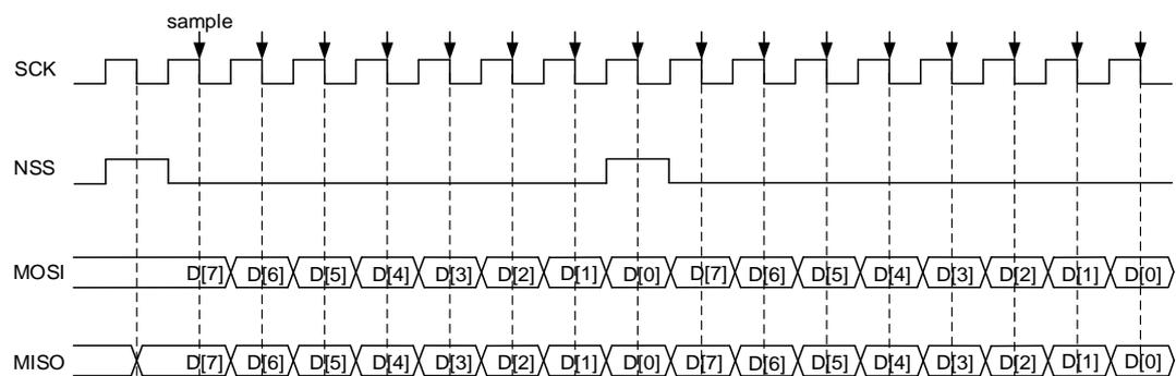
In master TI mode, SPI can perform continuous or non-continuous transfer. If the master writes SPI\_DATA register fast enough, the transfer is continuous, otherwise non-continuous. In non-continuous transfer there is an extra header clock cycle before each byte. While in continuous transfer, the extra header clock cycle only exists before the first byte and the following bytes' header clock is overlaid at the last bit of pervious bytes.
