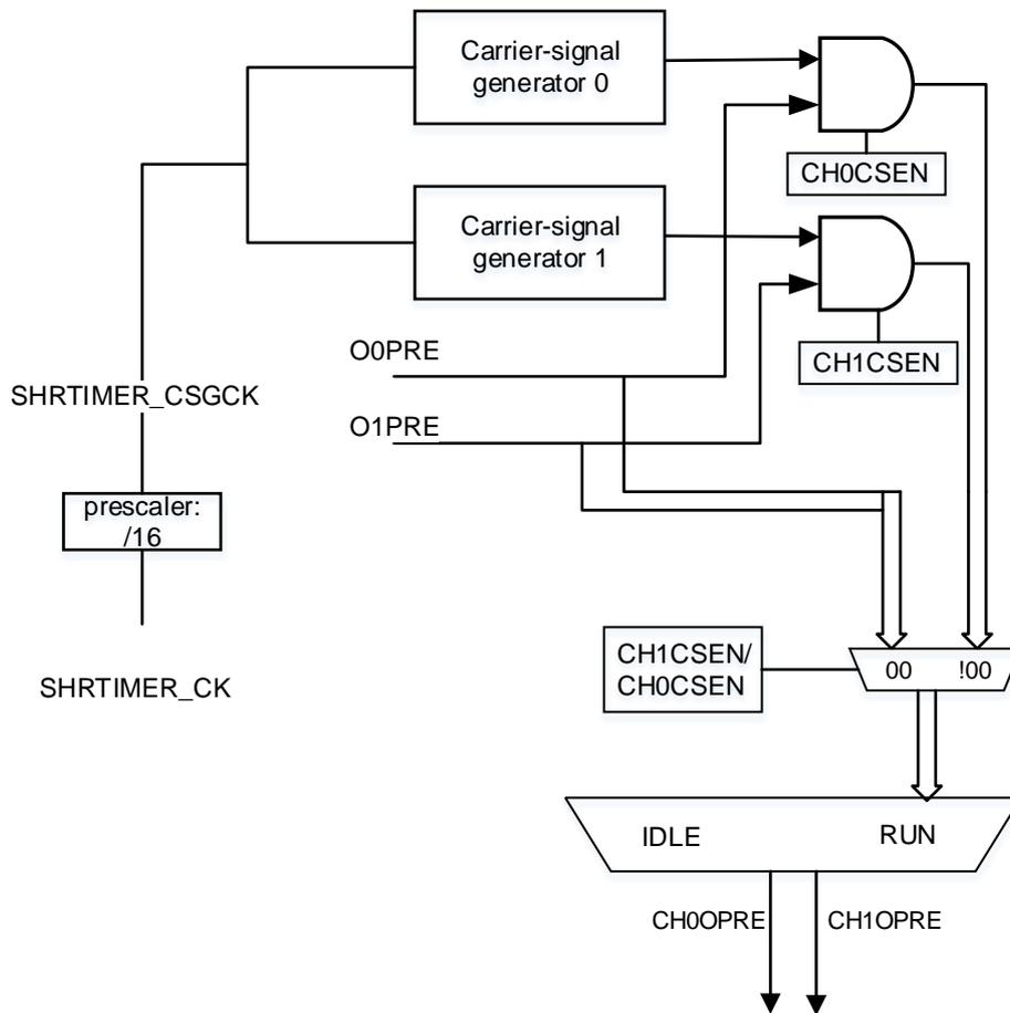
In carrier-signal mode, it is possible to define a specific pulse width before the beginning of the carrier-signal. The frequency and duty cycle of the carrier-signal are configurable. Refer to [Figure 19-37. SHRTIMER output with carrier-signal mode enabled.](#)
