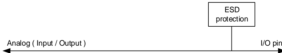
Figure 6-4. Basic structure of Analog configuration
