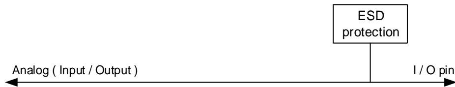
Figure 7-4. Basic structure of Analog configuration
