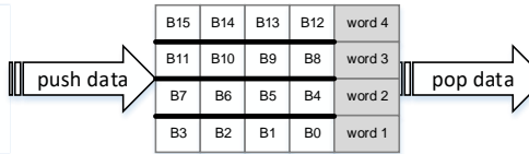
Figure 10-4. Data packing/unpacking when PWIDTH = '00'
