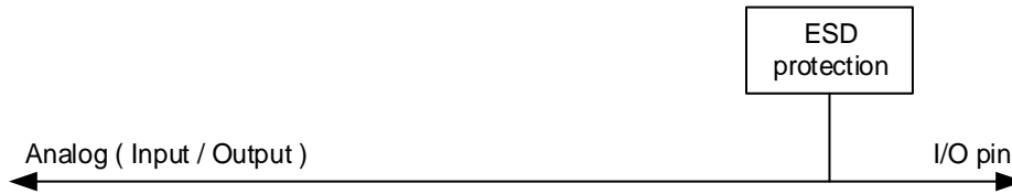
Figure 8-4. Basic structure of Analog configuration
