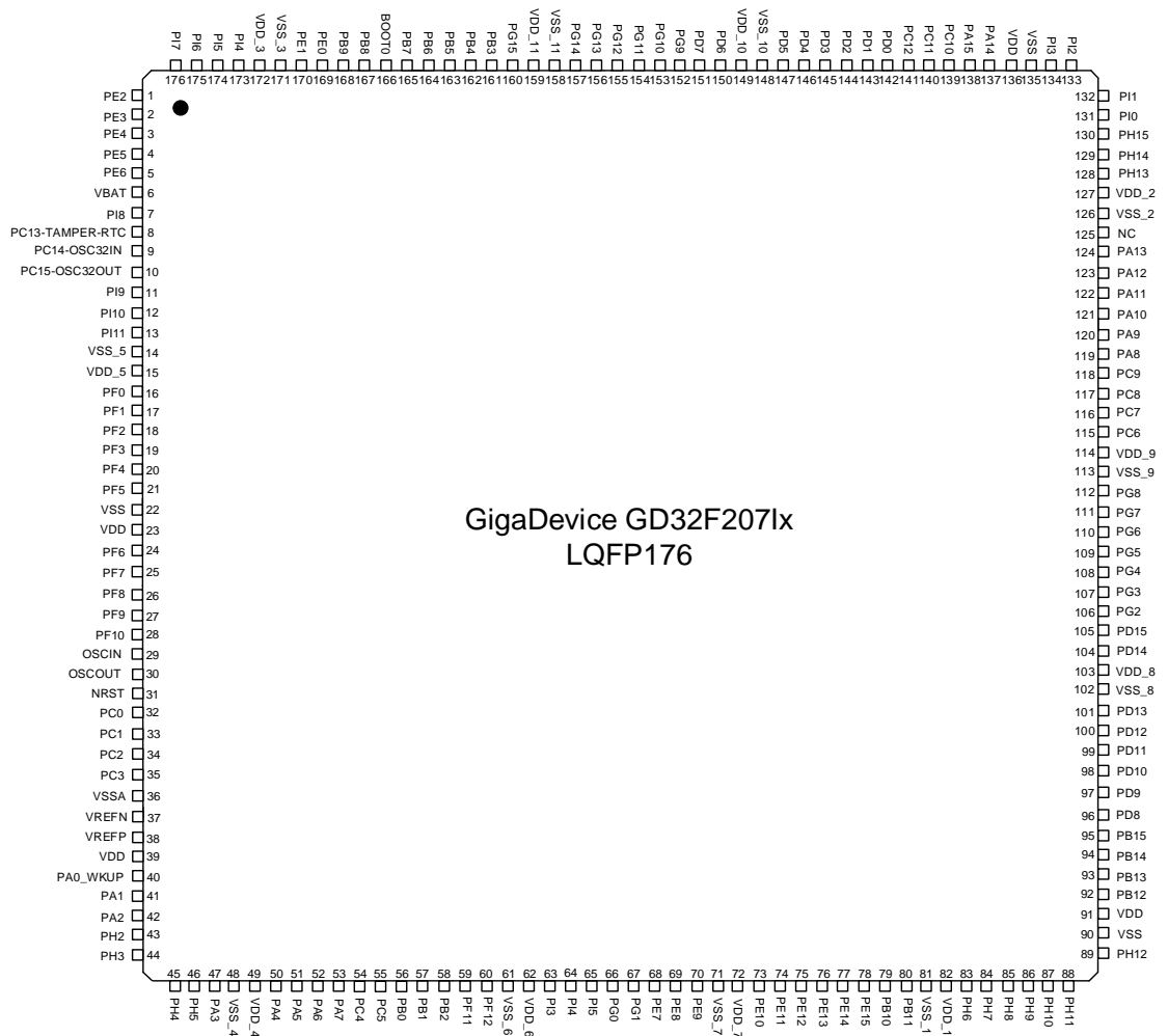
Figure 2-2. GD32F2071x LQFP176 pinouts
