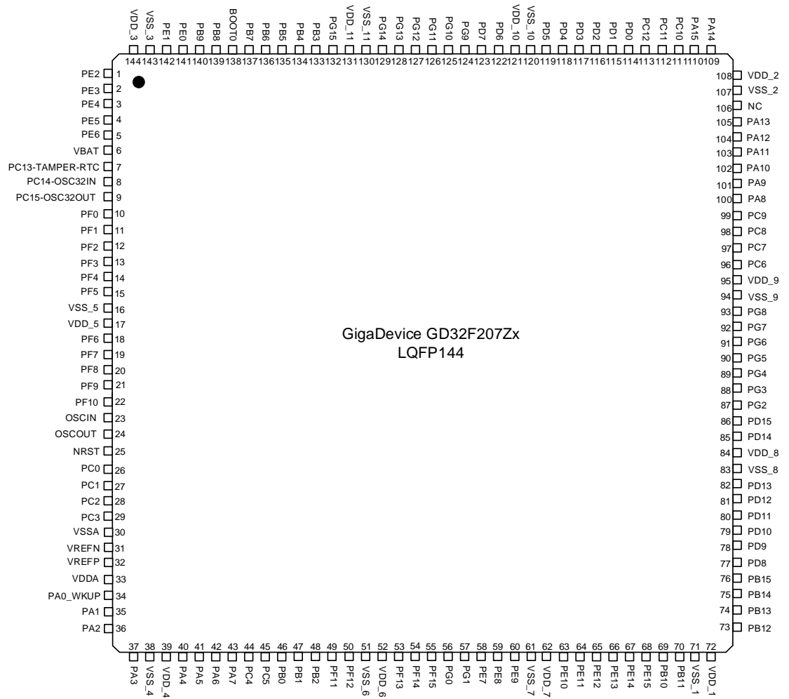
Figure 2-3. GD32F207Zx LQFP144 pinouts
