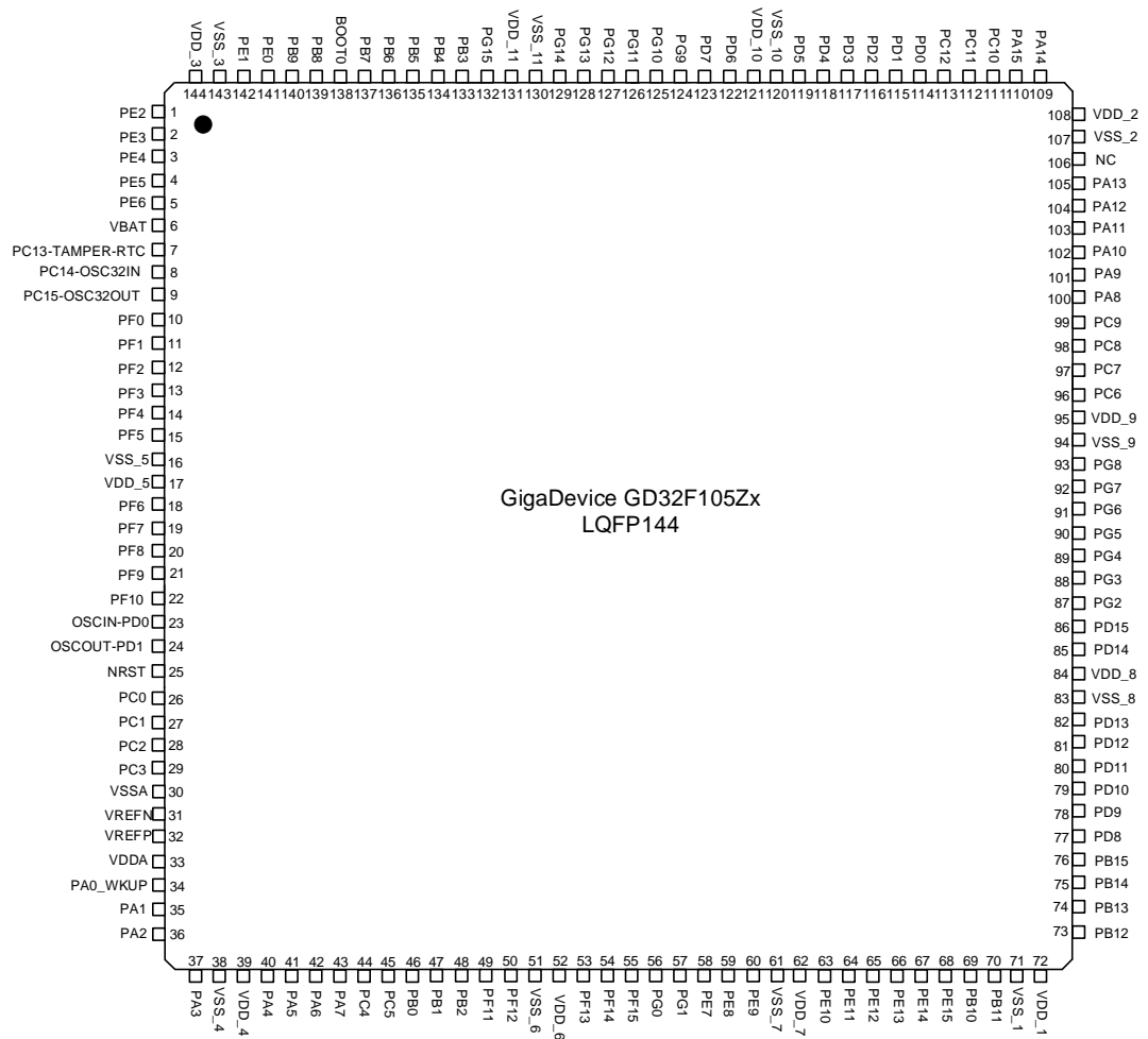
Figure 2-2. GD32F105Zx LQFP144 pinouts
