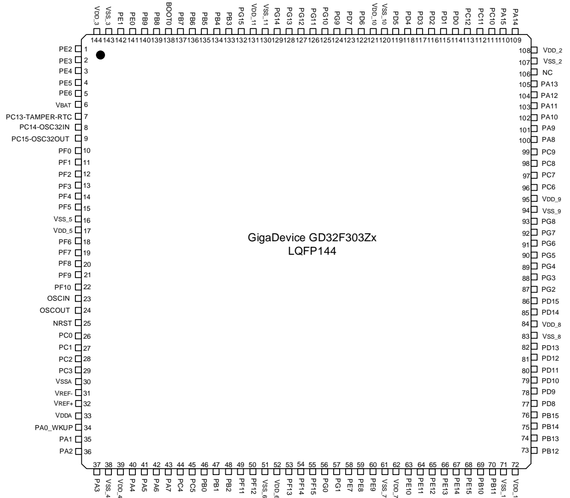
Figure 2-2. GD32F303Zx LQFP144 pinouts
