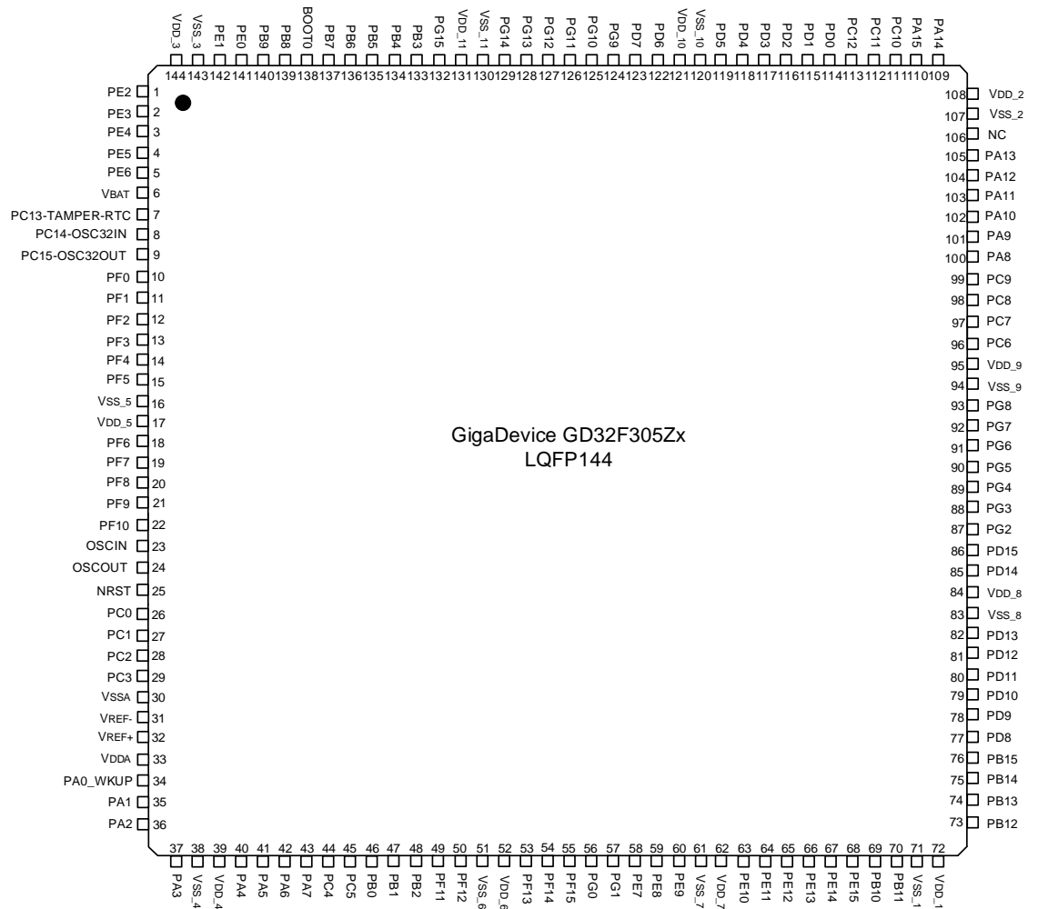
Figure 2-2. GD32F305Zx LQFP144 pinouts
