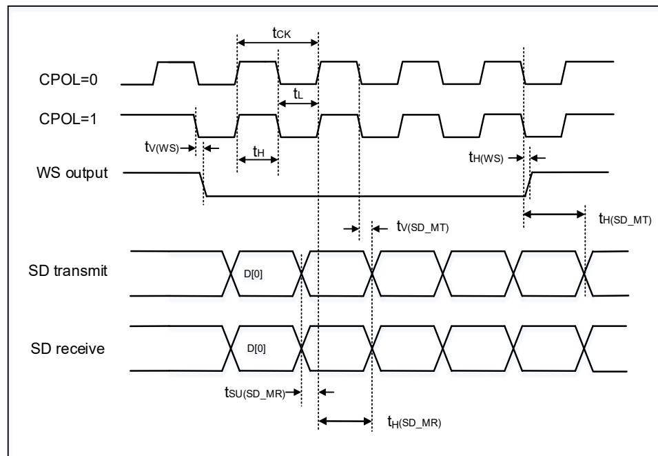
Figure 4-9. I2S timing diagram - slave mode
