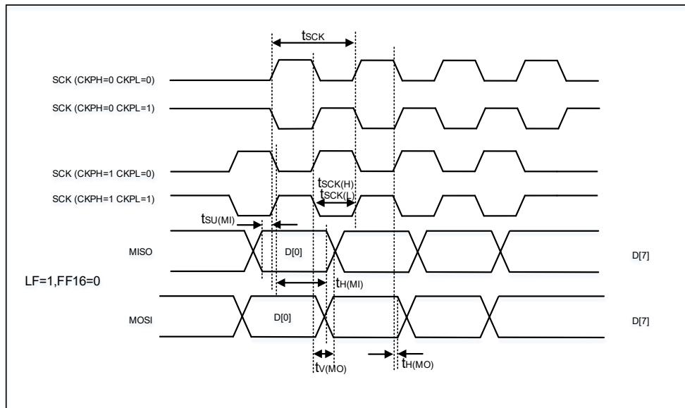
**Figure 4-7. SPI timing diagram - slave mode**
