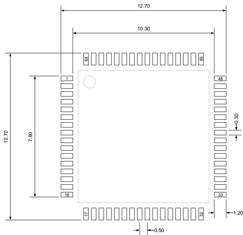
(Original dimensions are in millimeters)
