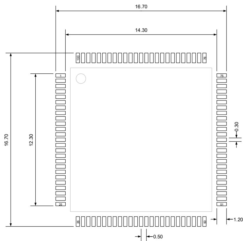
(Original dimensions are in millimeters)
