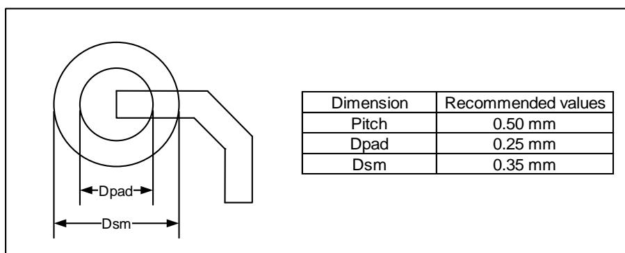
(Original dimensions are in millimeters)
