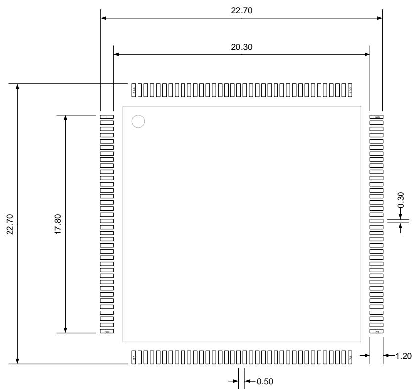
(Original dimensions are in millimeters)
