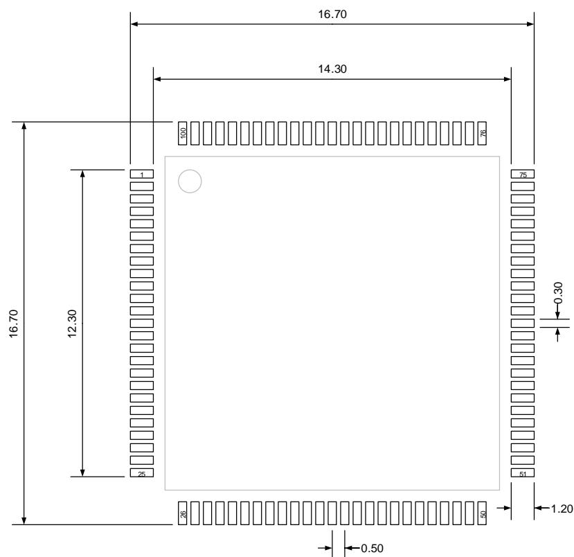
(Original dimensions are in millimeters)
