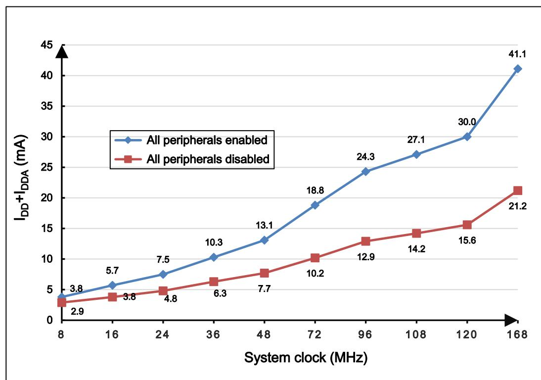
Figure 4-3. Typical supply current consumption in Sleep mode
