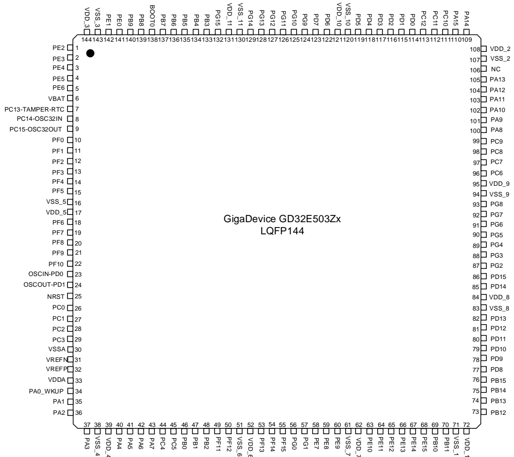
Figure 2-2. GD32E503Zx LQFP144 pinouts
