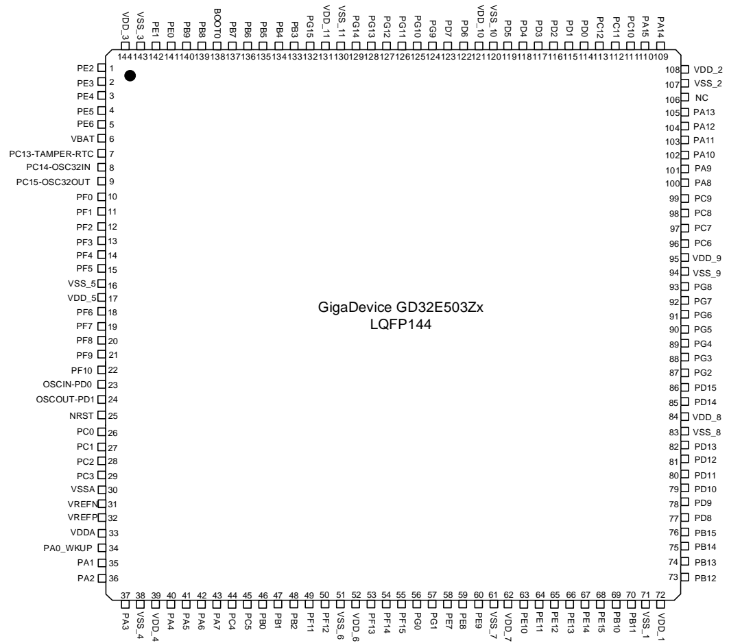
Figure 2-2. GD32E503Zx LQFP144 pinouts
