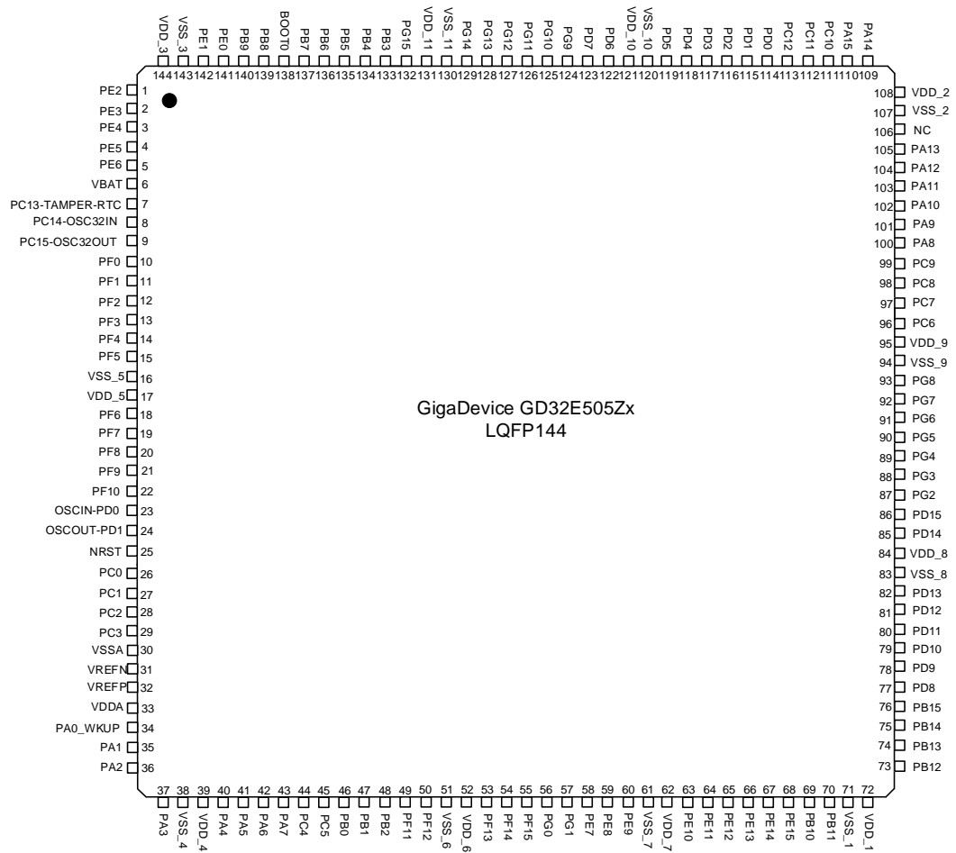
Figure 2-2. GD32E505Zx LQFP144 pinouts
