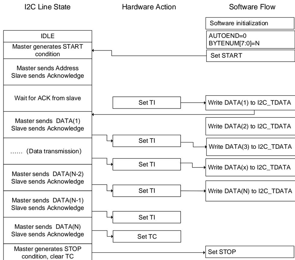
**Figure 22-19. Programming model for master transmitting (N>255)**
