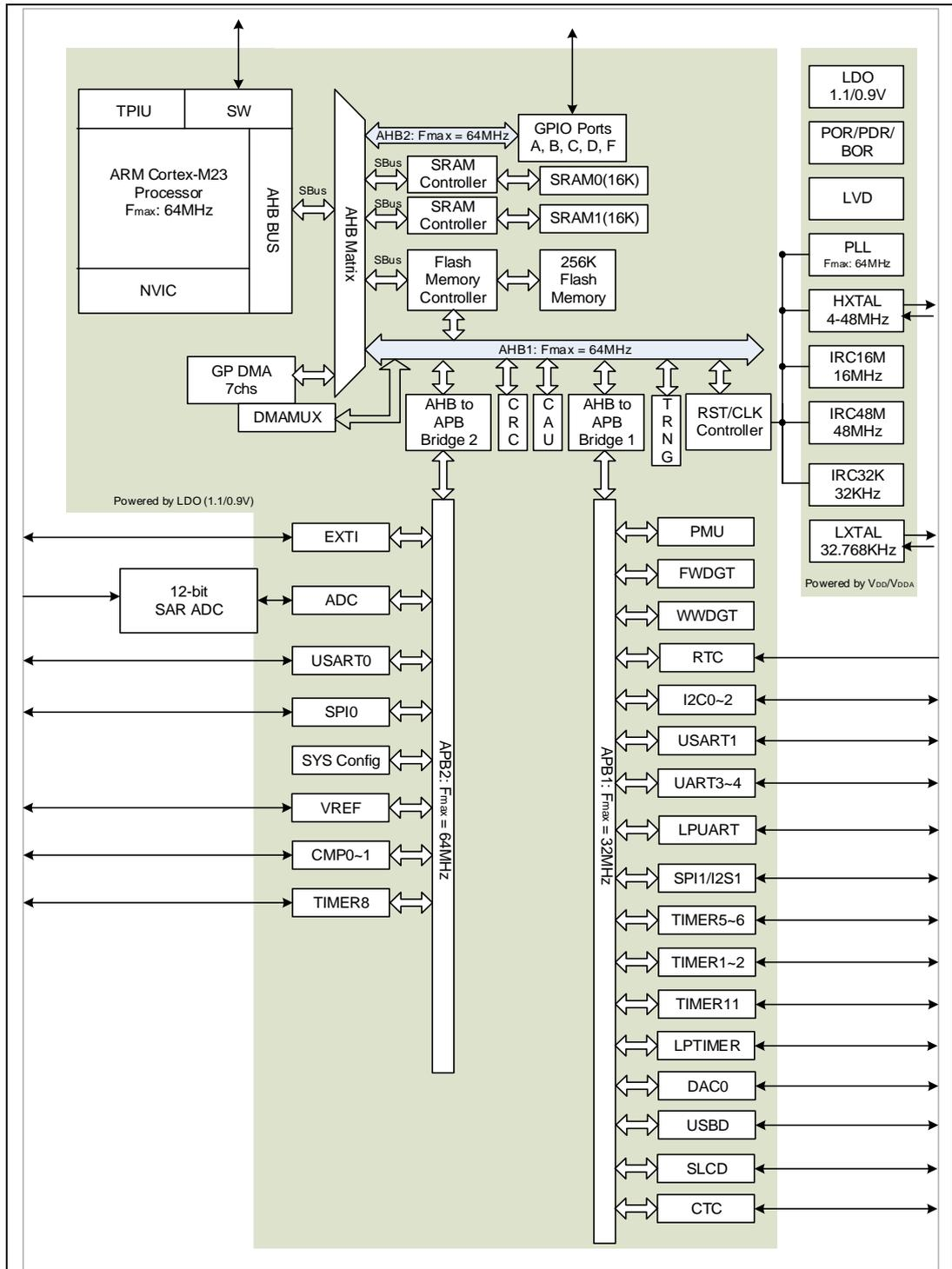
**Figure 1-3. Series system architecture of GD32L23x(x=5) series**
