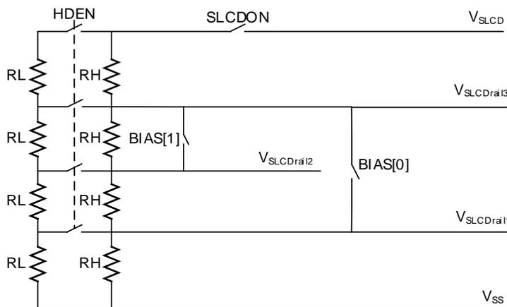
During the transitions, the low value resistors ( $R_L$ ) are switched on to increase the current in order to quickly reach the static state. Then the low value resistors ( $R_L$ ) are switched off, the high value resistors ( $R_H$ ) are used to reduce the power. The length of the time during  $R_L$  is switched on depend on the PULSE[2:0] bits in the SLCD\_CFG register. The  $R_L$  can be always switched on according to setting the HDEN bit in the SLCD\_CFG register.
