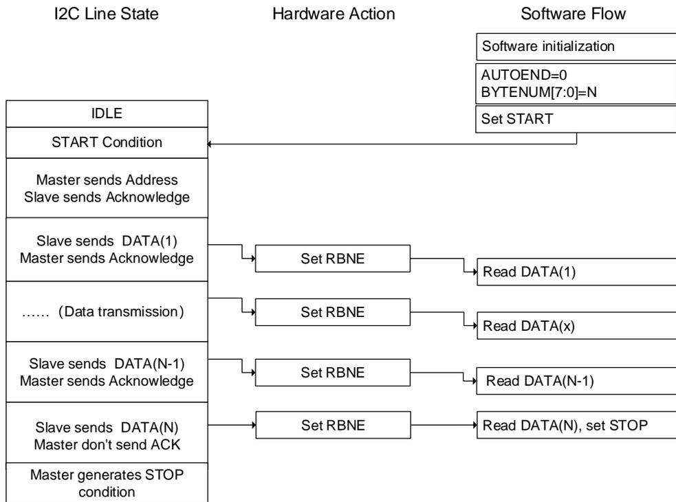
**Figure 22-21. Programming model for master receiving (N>255)**
