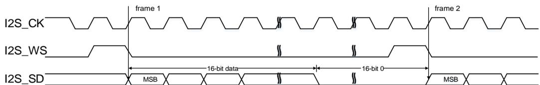
The timing diagrams for each configuration of the long frame synchronization mode are shown below.
