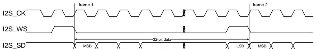
**Figure 23-42. PCM standard short frame synchronization mode timing diagram**
