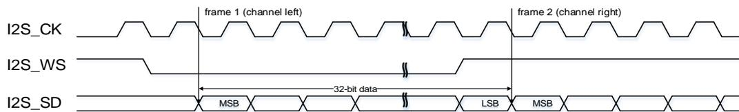
**Figure 23-21. I2S Phillips standard timing diagram (DTLEN=10, CHLEN=1, CKPL=1)**
