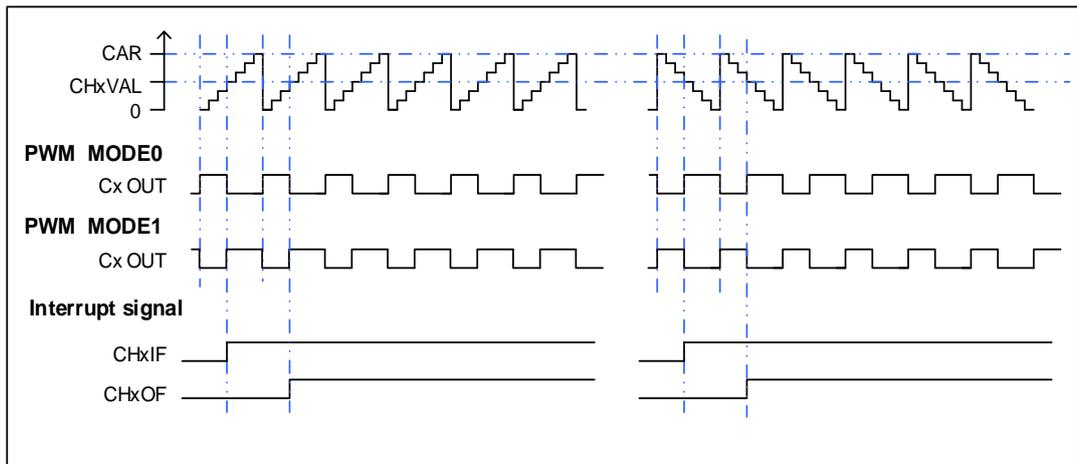
**Figure 18-17. Timing chart of CAPWM**
