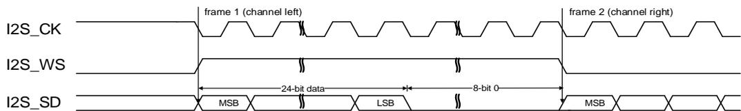
**Figure 23-32. MSB justified standard timing diagram (DTLEN=00, CHLEN=1, CKPL=0)**
