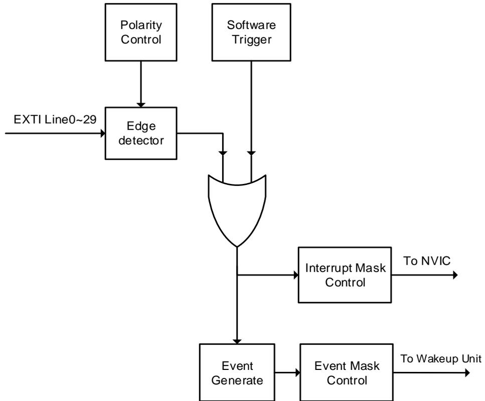
Figure 6-2. Block diagram of EXTI for GD32L235xx devices
