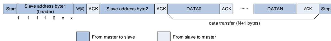
**Figure 22-5. I2C communication flow with 7-bit address (Master Transmit)**
