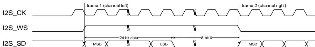
**Figure 23-31. MSB justified standard timing diagram (DTLEN=01, CHLEN=1, CKPL=1)**
