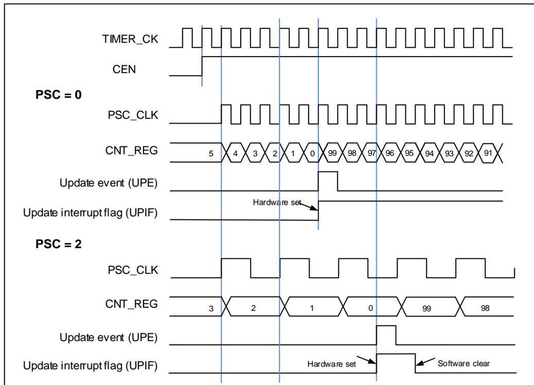
Figure 18-40. Timing chart of down counting mode, change TIMERx\_CAR ongoing
