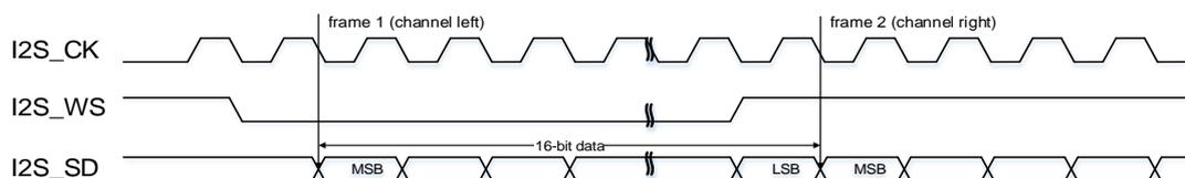
**Figure 23-19. I2S Phillips standard timing diagram (DTLEN=00, CHLEN=0, CKPL=1)**
