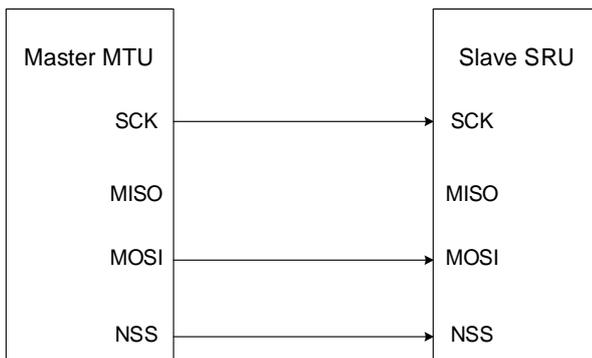
**Figure 23-10. A typical bidirectional connection**
