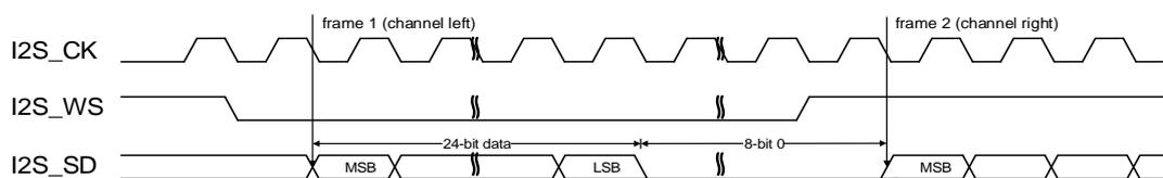
**Figure 23-23. I2S Phillips standard timing diagram (DTLEN=01, CHLEN=1, CKPL=1)**
