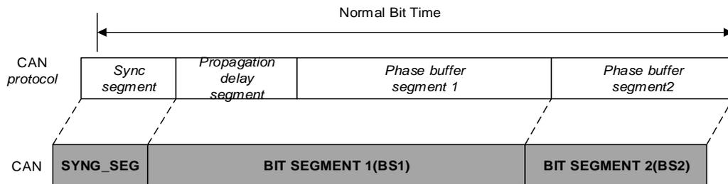
The resynchronization Jump Width (SJW): it can be lengthened or shortened to compensate for the Synchronization error of the CAN network node. It is programmable from 1 to 4 time quanta.
