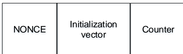
Figure 10-12. Counter block structure
