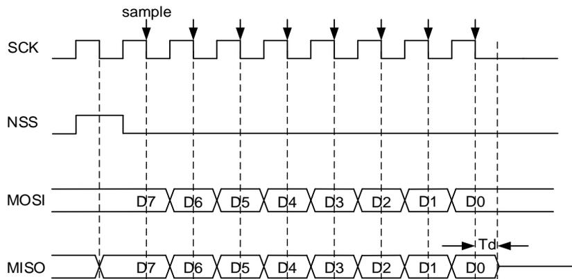
In slave TI mode, after the last rising edge of SCK in transfer, the slave begins to transmit the LSB bit of the last data byte, and after a half-bit time, the master begins to sample the line. To make sure that the master samples the right value, the slave should continue to drive this bit after the falling sample edge of SCK for a period of time before releasing the pin. This time is called  $T_d$ .  $T_d$  is decided by PSC [2:0] bits in SPI\_CTL0 register.
