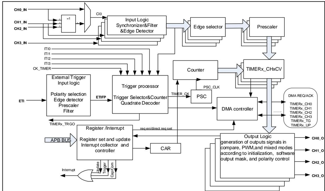
Figure 18-33. General Level 0 timer block diagram for GD32L235 provides details on the internal configuration of the general level0 timer.
