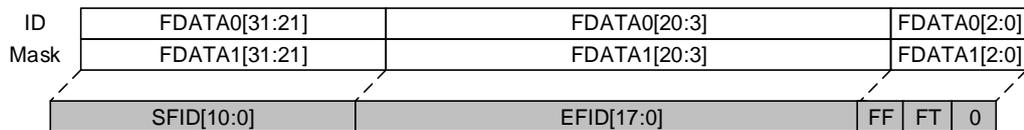
**Figure 27-8. 16-bit mask mode filter**
