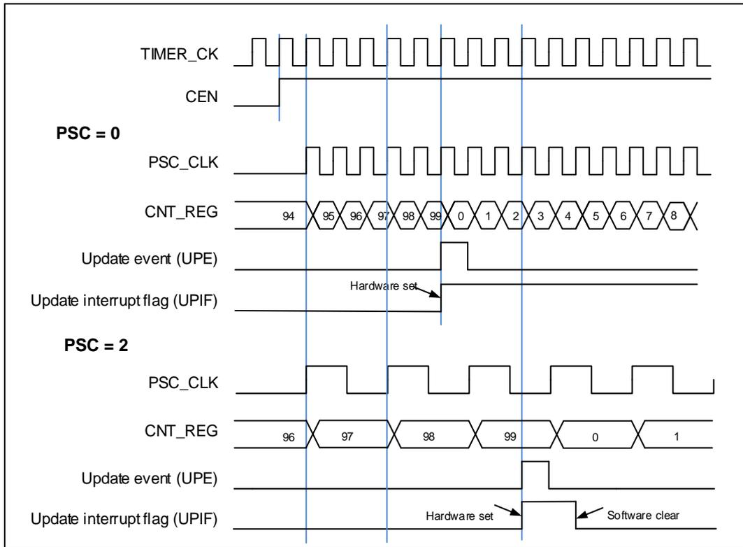
Figure 18-38. Timing chart of up counting, change TIMERx\_CAR ongoing
