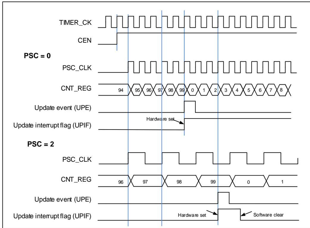
Figure 18-62. Up-counter timechart, change TIMERx\_CAR on the go
