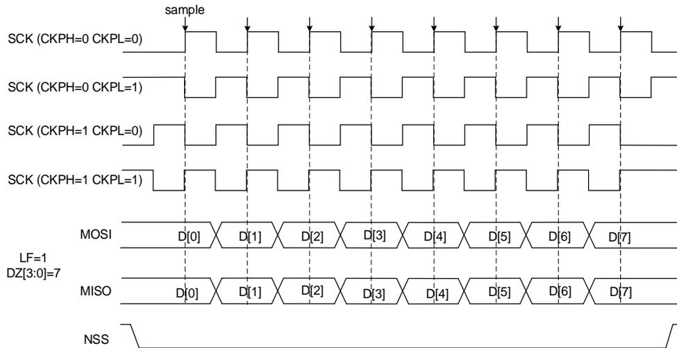
Figure 23-3. SPI0 data frame right-aligned diagram
