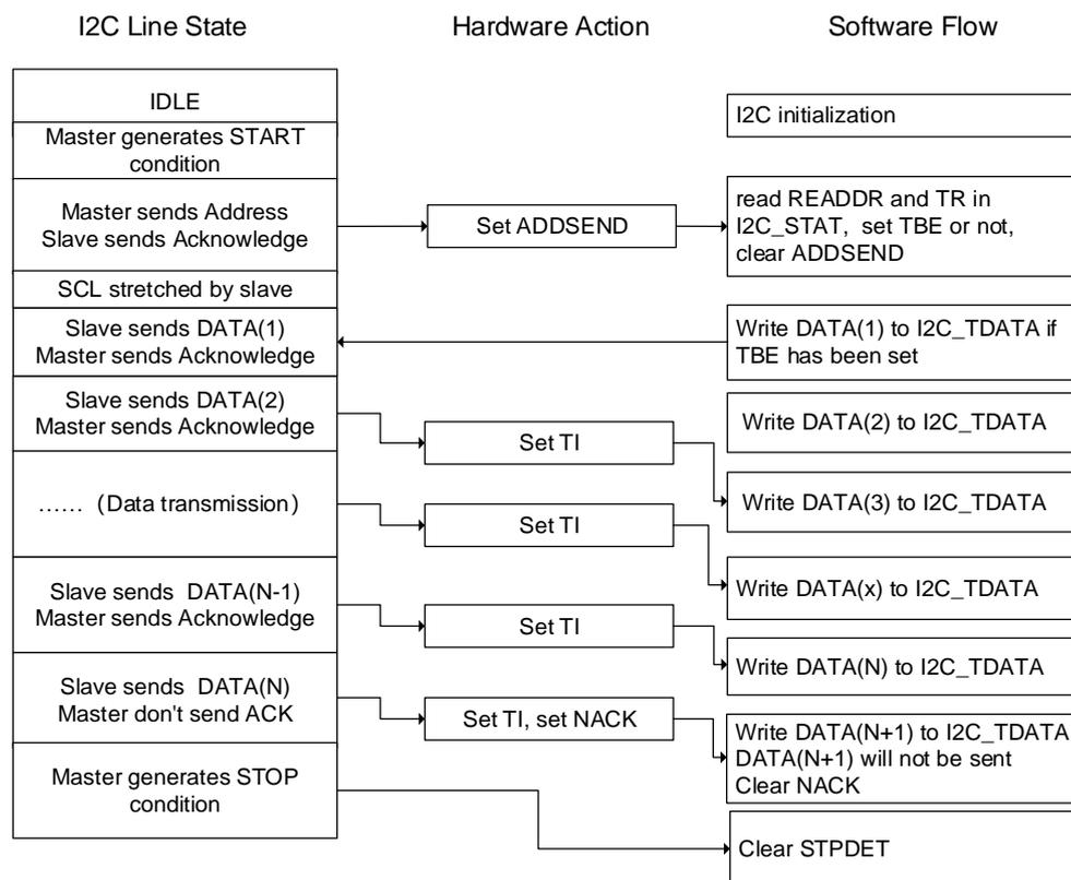
Figure 22-15. Programming model for slave transmitting when SS=1
