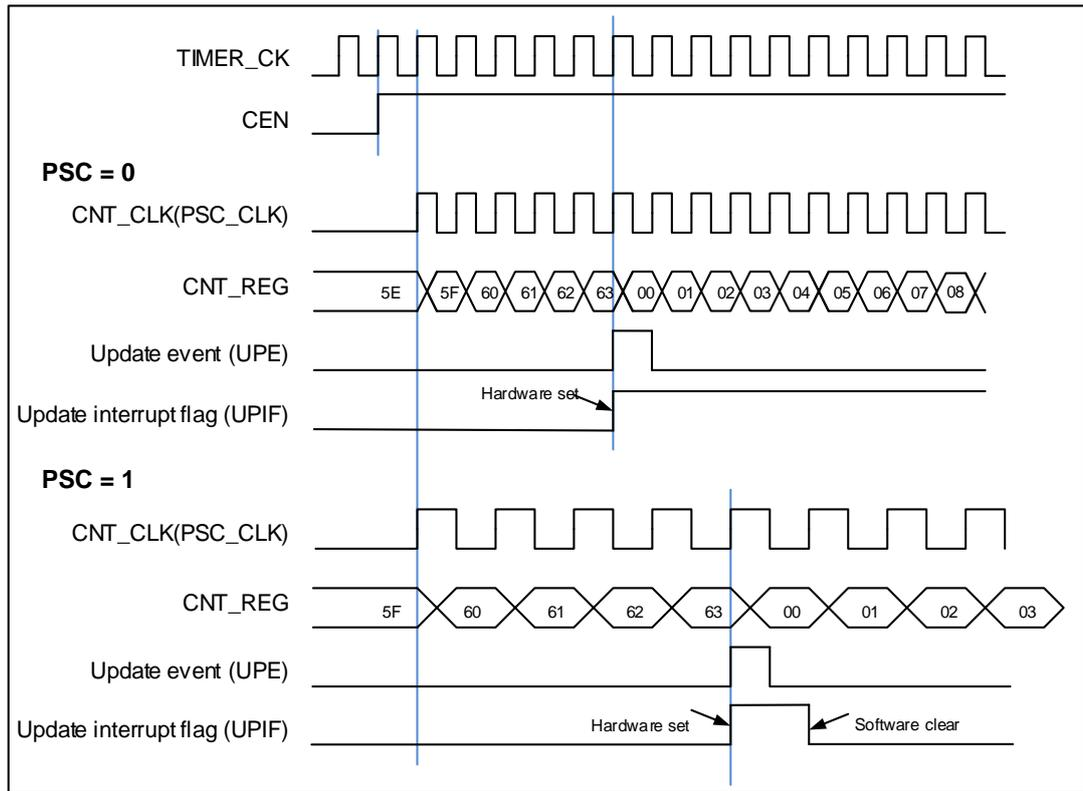
Figure 18-78. Up-counter timechart, change TIMERx\_CAR ongoing
