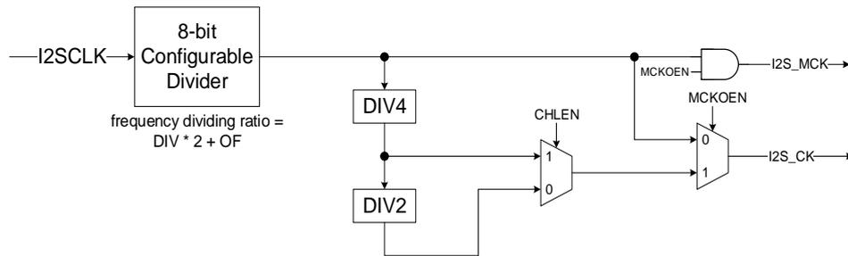
The block diagram of I2S clock generator is shown as [Figure 23-54. Block diagram of I2S clock generator](#). The I2S interface clocks are configured by the DIV bits, the OF bit, the MCKOEN bit in the SPI\_I2SPSC register and the CHLEN bit in the SPI\_I2SCTL register. The source clock is the system clock(CK\_SYS). The I2S bitrate can be calculated by the formulas shown in [Table 23-7. I2S bitrate calculation formulas](#).
