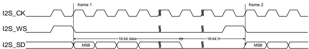
**Figure 23-45. PCM standard short frame synchronization mode timing diagram (DTLEN=00, CHLEN=1, CKPL=1)**
