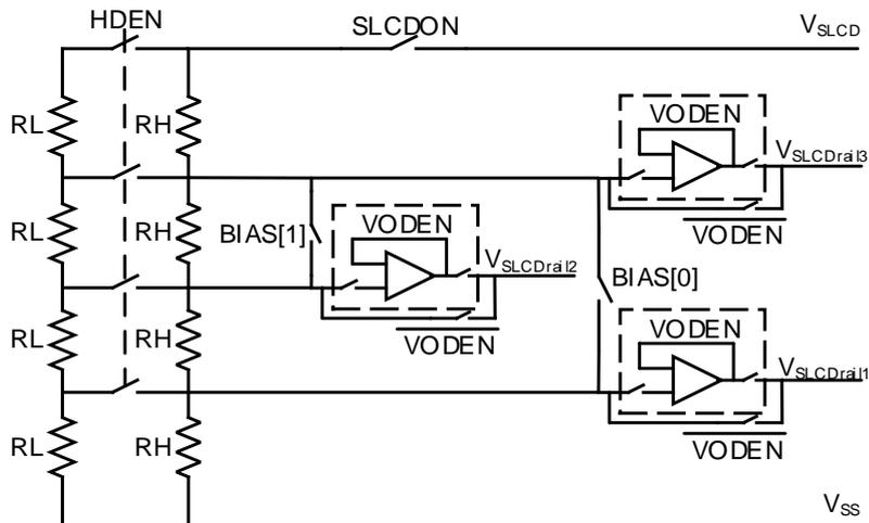
Figure 25-6. SLCD Resist divider network for GD32L235 series
