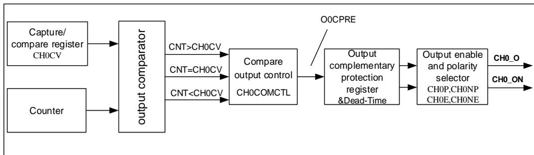
**Figure 18-82. Output compare logic (CH1\_O)**
