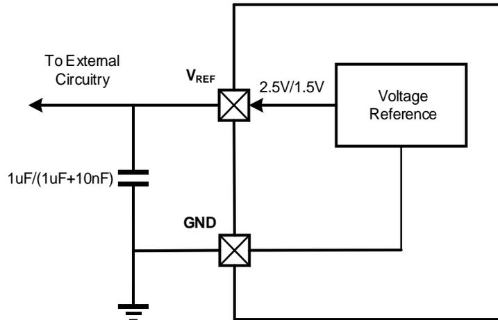
The internal reference voltage can be configured in four different modes depending on VREFEN and HIPM bits configuration. These modes are provided in the table below:
