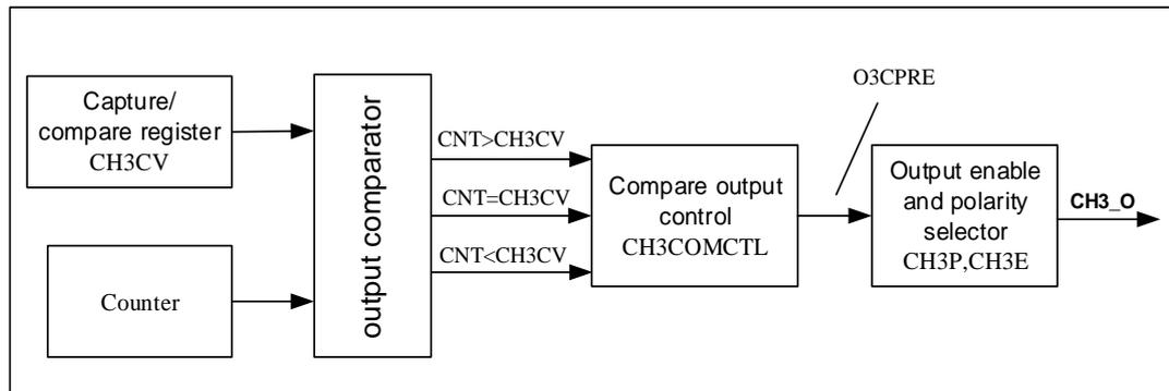
[Figure 18-13. Output compare logic \(with complementary output, x=0,1,2\)](#) and
