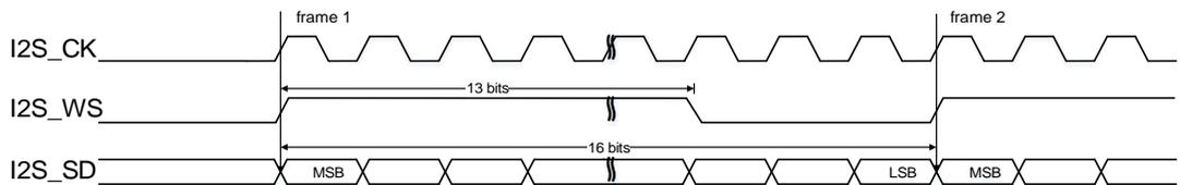
**Figure 23-47. PCM standard long frame synchronization mode timing diagram**
