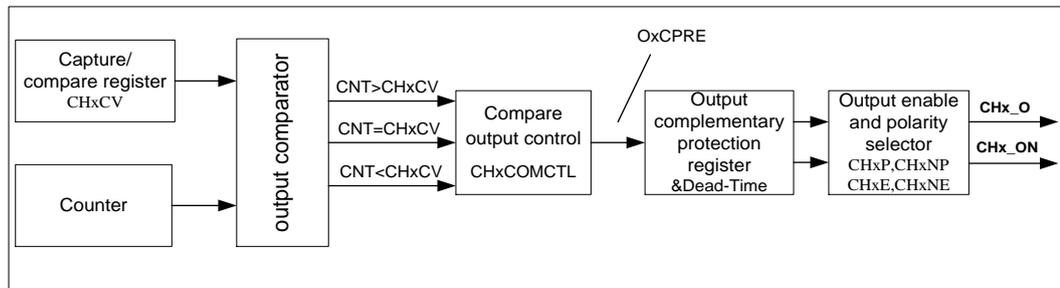
**Figure 18-14. Output compare logic (CH3\_O)**
