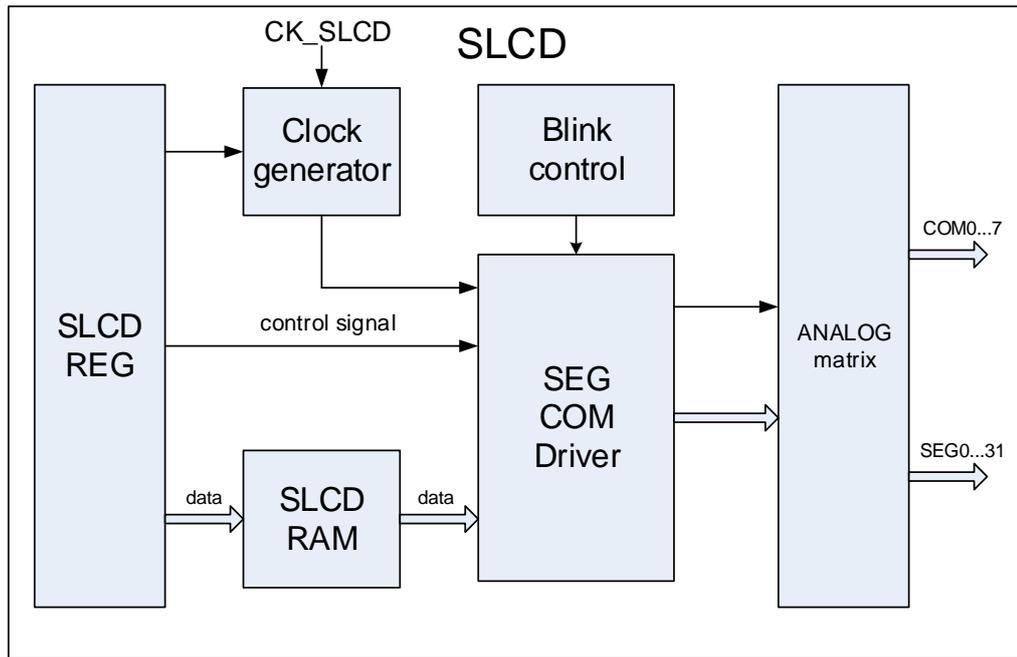
The SLCD REG is the register of SLCD controller, which configured by APB bus, and generate interrupt to CPU. It includes SLCD\_CTL, SLCD\_CFG, SLCD\_STAT, SLCD\_STATC, SLCD\_DATAx registers.
