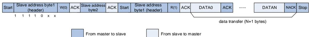
**Figure 22-8. I2C communication flow with 10-bit address (Master Receive when HEAD10R=1)**
