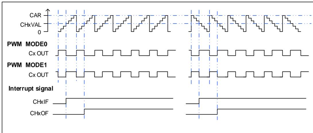
Figure 18-46. Timing chart of CAPWM
