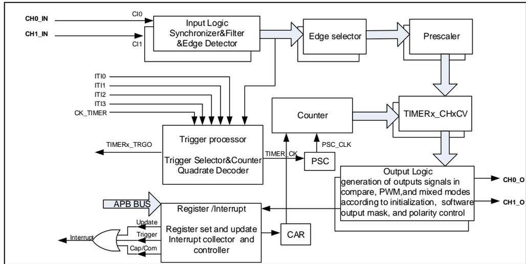
[Figure 18-57. General Level 1 timer block diagram for GD32L235](#) provides details on the internal configuration of the general level1 timer.
