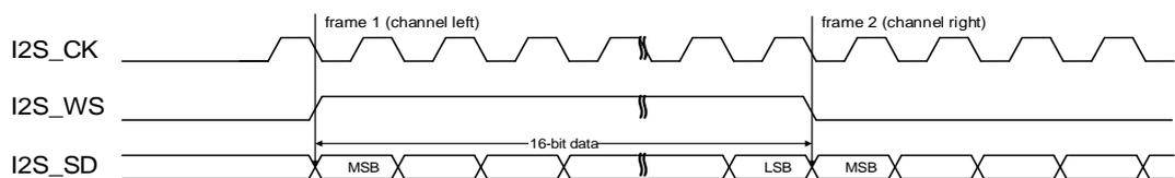
**Figure 23-27. MSB justified standard timing diagram (DTLEN=00, CHLEN=0, CKPL=1)**
