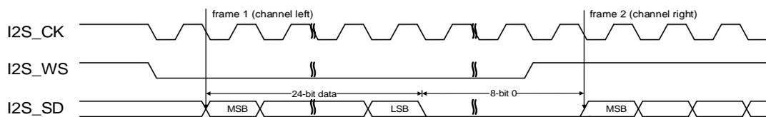
When the packet type is 24-bit data packed in 32-bit frame, two write or read operations to or from the SPI\_DATA register are needed to complete a frame. In transmission mode, if a 24-
