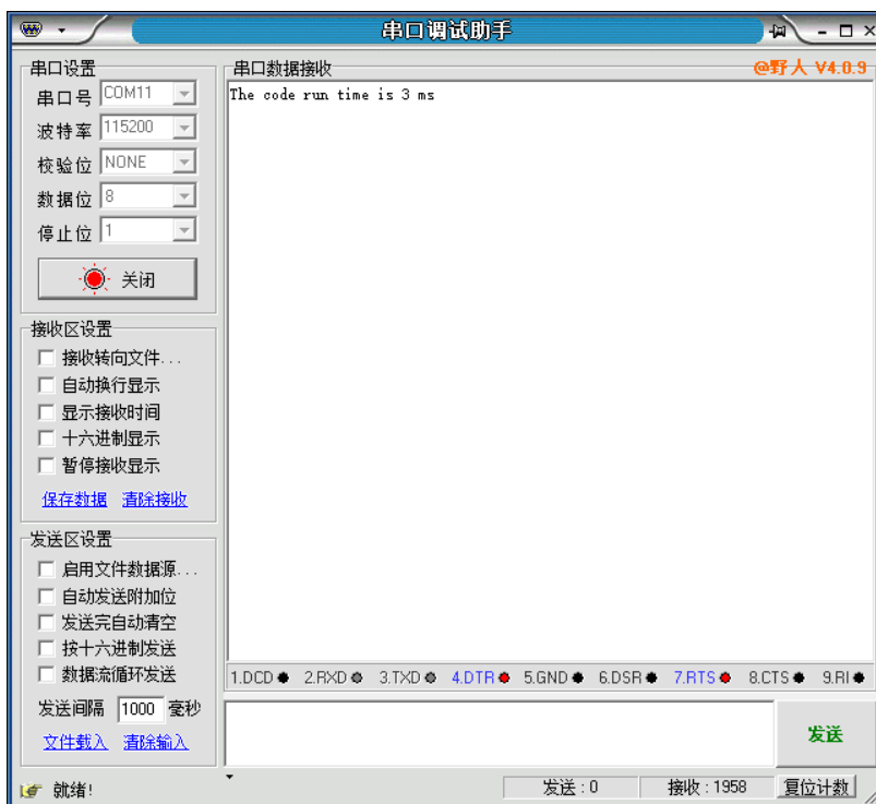
Figure 2-2. SysTick measurement code running time result printing
