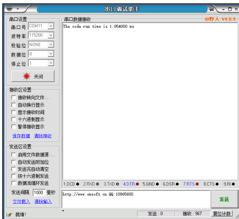
Figure 2-1. Timer 1 measures the running time of the code and prints the result
