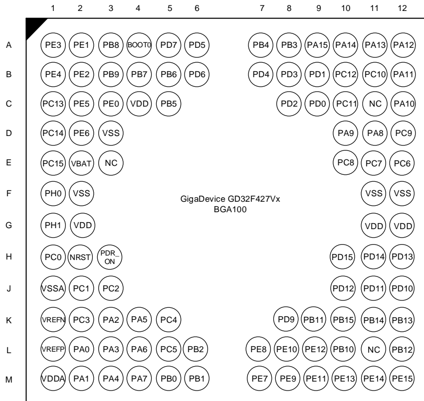
Figure 2-3. GD32F427Vx BGA100 pinouts
