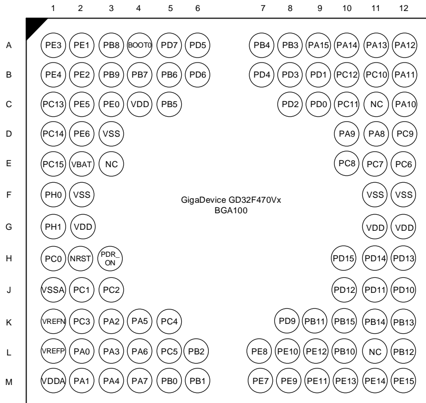
Figure 2-4. GD32F470Vx BGA100 pinouts
