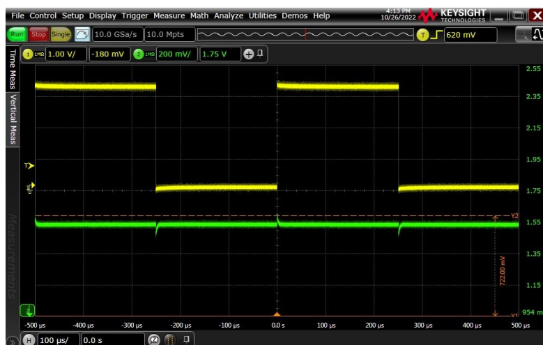
Figure 2-8. The waveform of crosstalk between analog I/O and digital I/O
