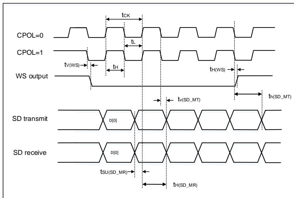
Figure 4-9. I2S timing diagram - slave mode
