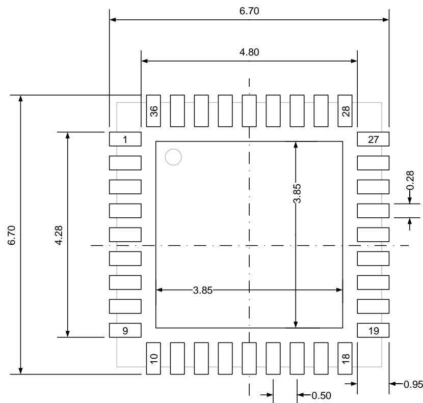
(Original dimensions are in millimeters)
