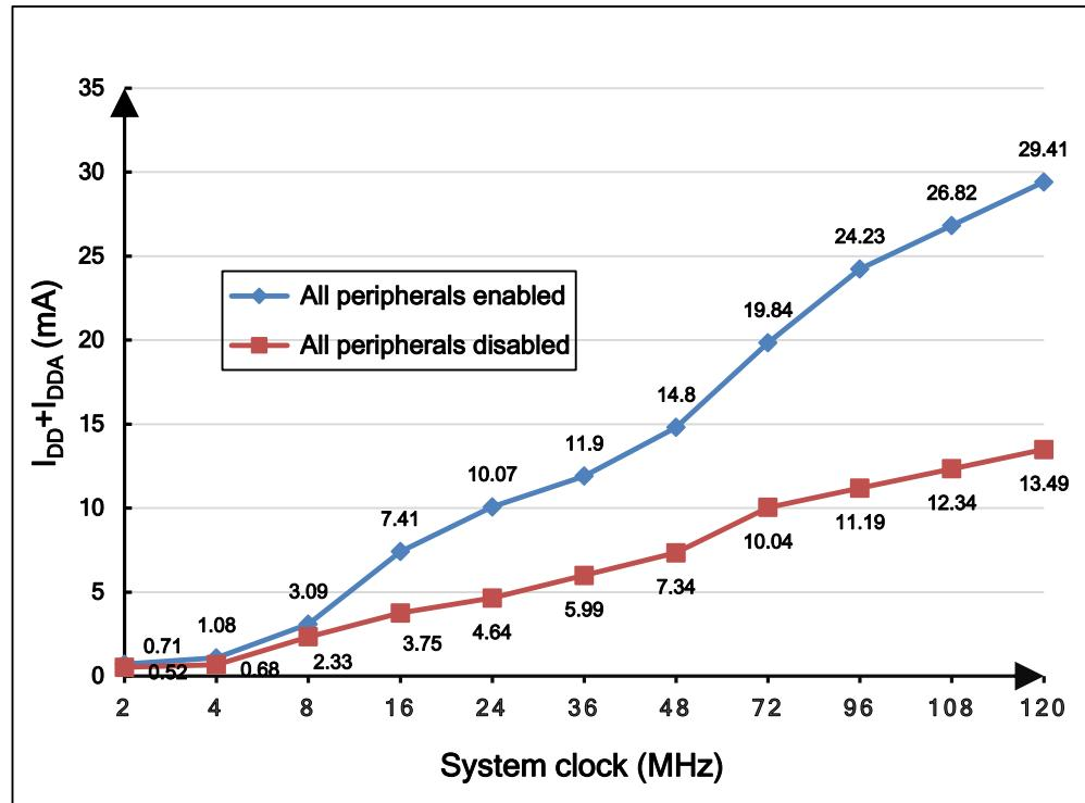
Figure 4-3. Typical supply current consumption in Sleep mode
