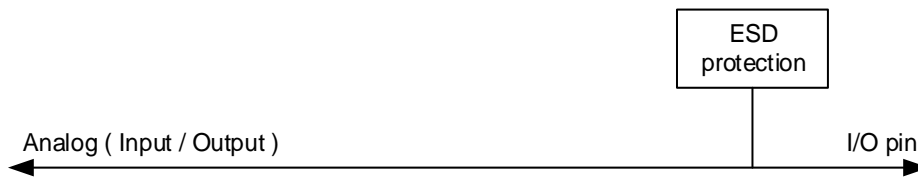
Figure 8-4. Basic structure of Analog configuration
