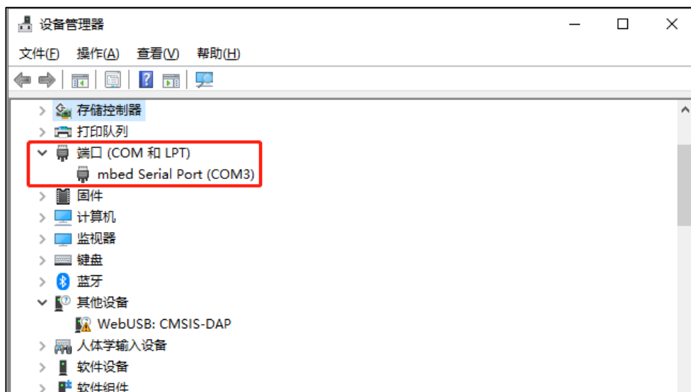
Figure 7-2. List of device manager serial ports
