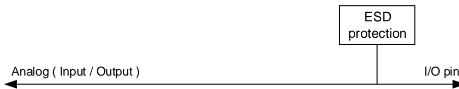
Figure 8-4. Basic structure of Analog configuration
