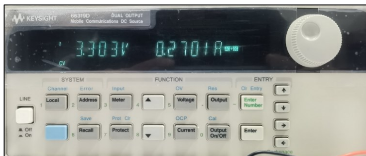
Figure 5-2. Tx power consumption test
