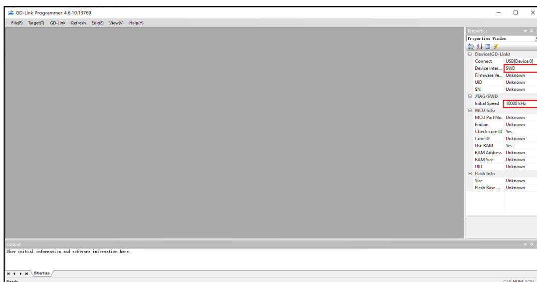
Figure 3-16. GD-Link programmer programming options configuration
