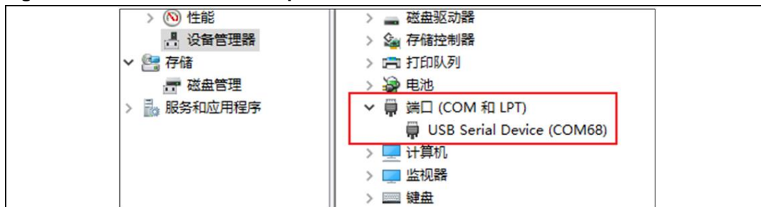
Figure 3-1. Installation of serial port drive
