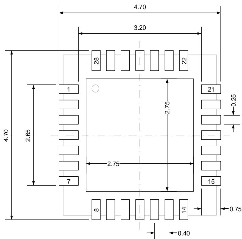
(Original dimensions are in millimeters)
