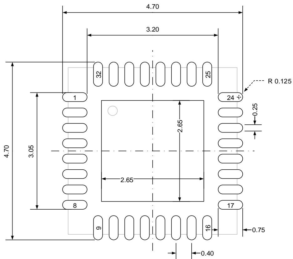
(Original dimensions are in millimeters)
