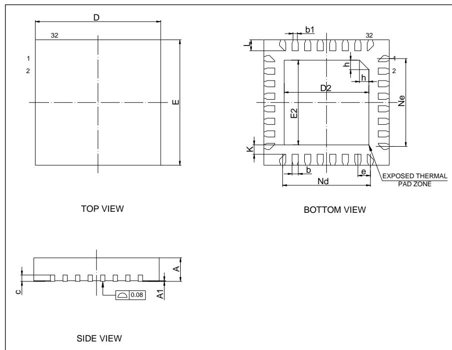
**Table 5-5. QFN32 4X4 mm,0.4 Pitch package dimensions**
