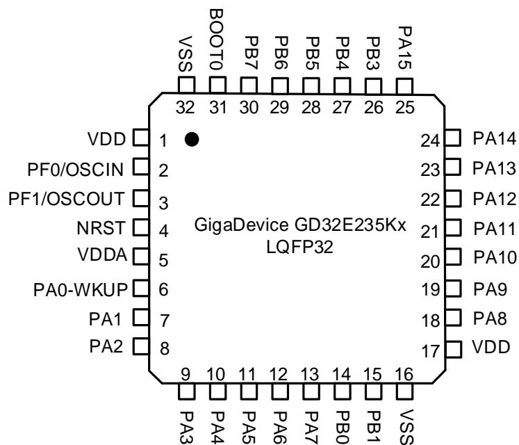
**Figure 2-5. GD32E235Kx QFN32 pinouts**
