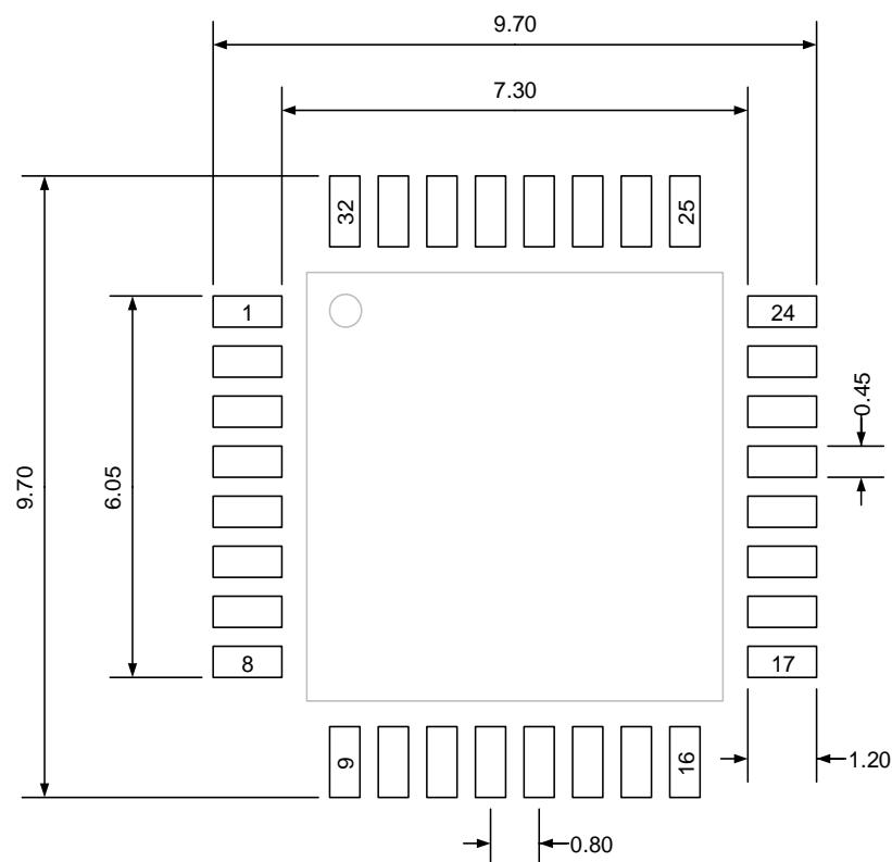
(Original dimensions are in millimeters)
