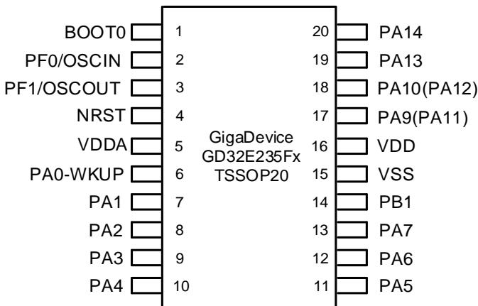
Figure 2-9. GD32E235Fx LGA20 pinouts
