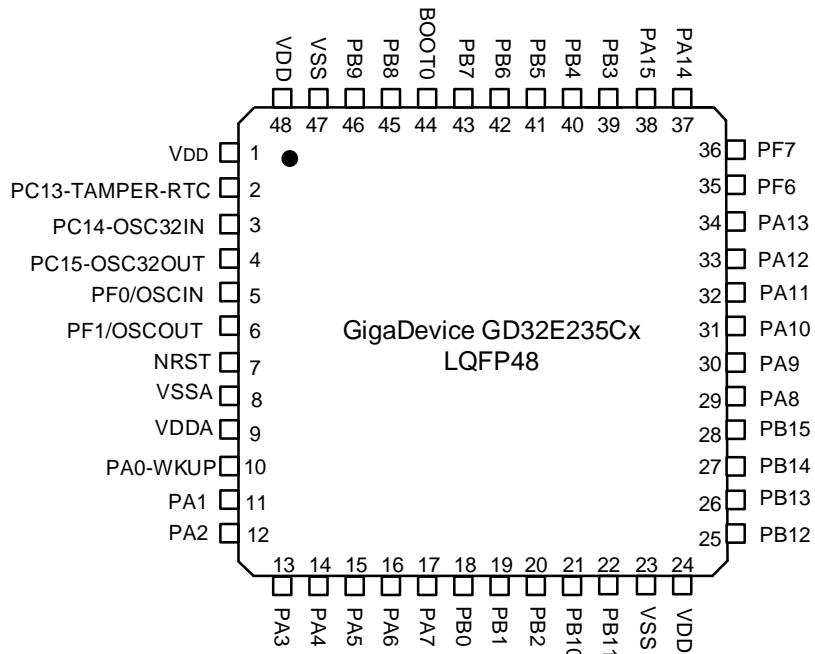
**Figure 2-3. GD32E235Cx QFN48 pinouts**
