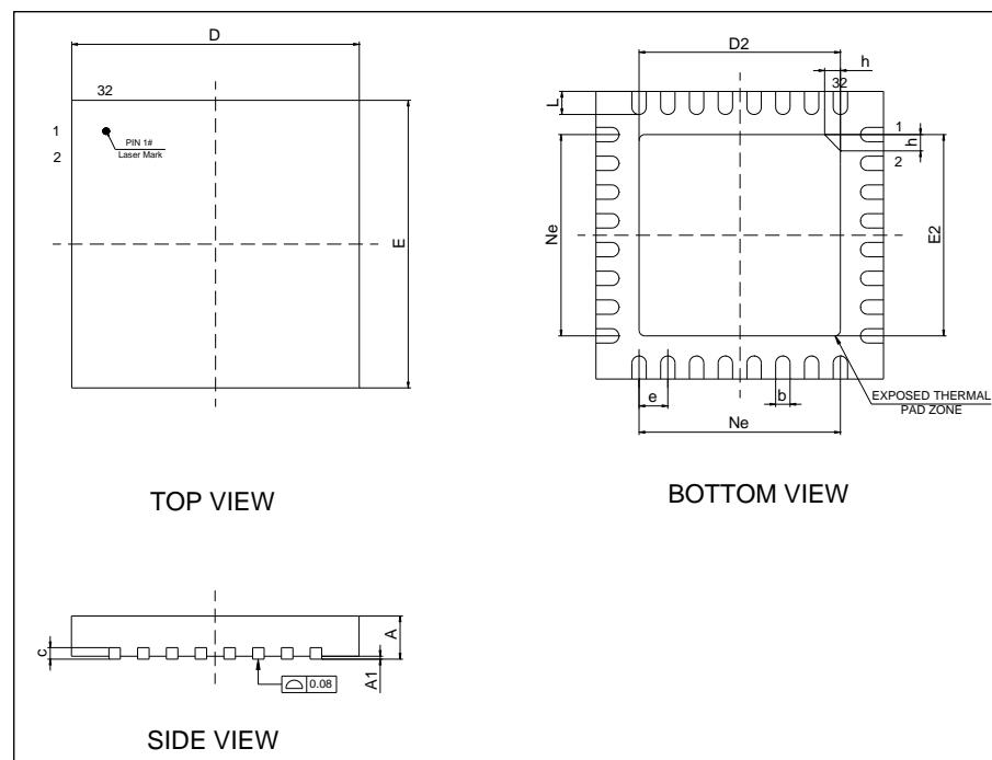
**Table 5-4. QFN32 5X5 mm,0.5 Pitch package dimensions**
