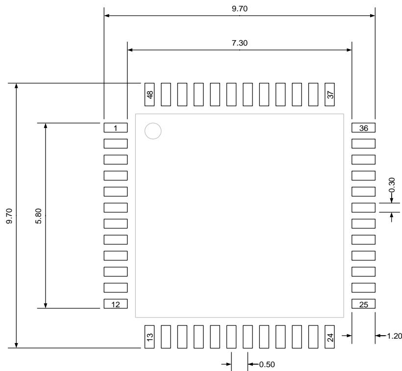
(Original dimensions are in millimeters)
