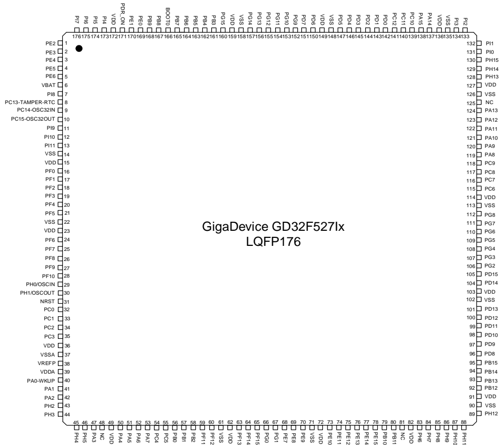
Figure 2-3. GD32F527Ix LQFP176 pinouts
