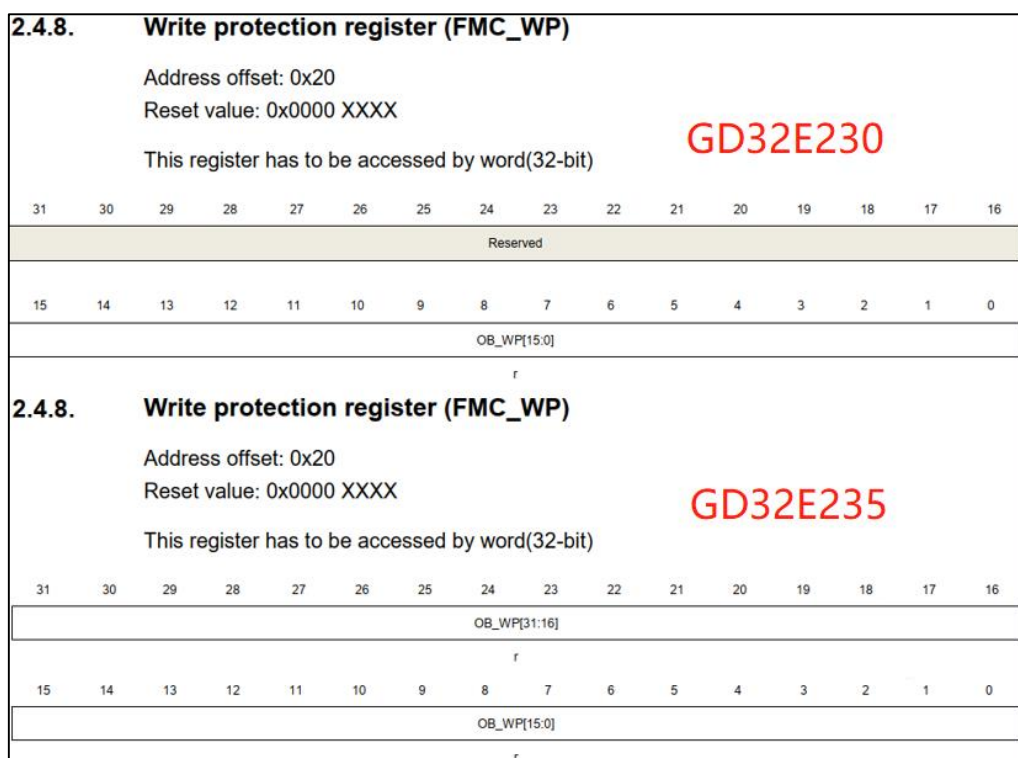
Figure 4- 1. Comparison of Write Protect Registers (FMC_WP) Differences between GD32E230xx and GD32E235xx devices
