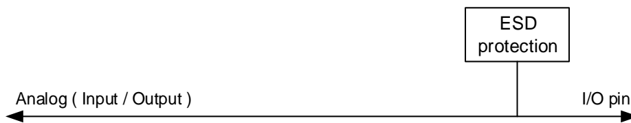
Figure 8-4. Basic structure of Analog configuration
