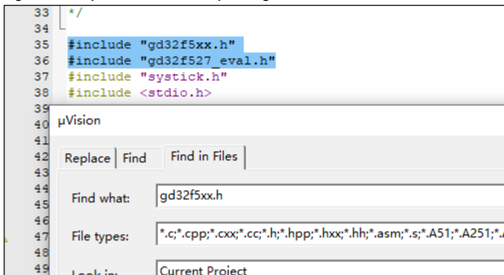
Figure 4-9. Replacement of corresponding header files
