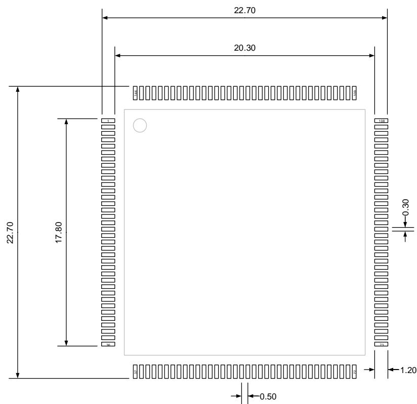
(Original dimensions are in millimeters)
