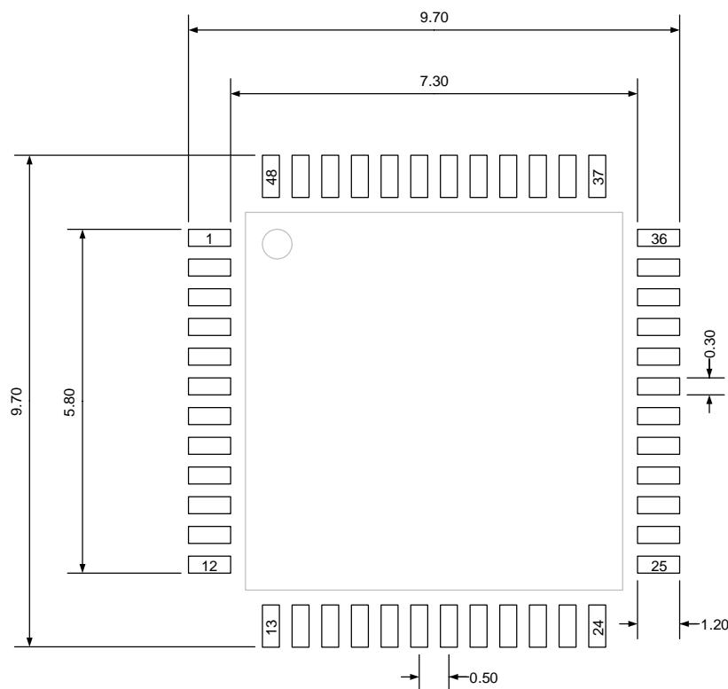
(Original dimensions are in millimeters)
