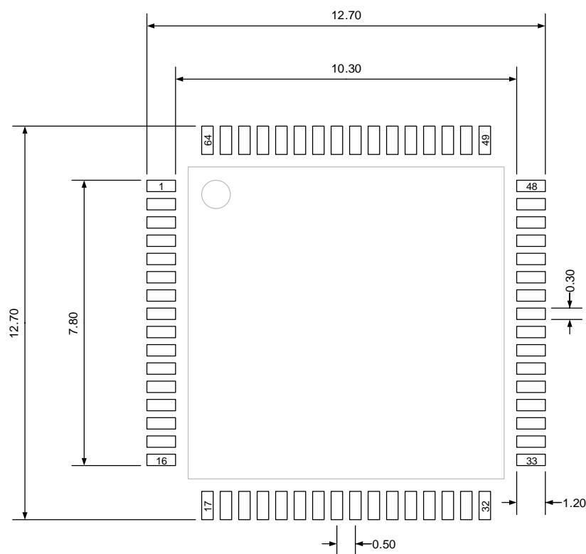
(Original dimensions are in millimeters)
