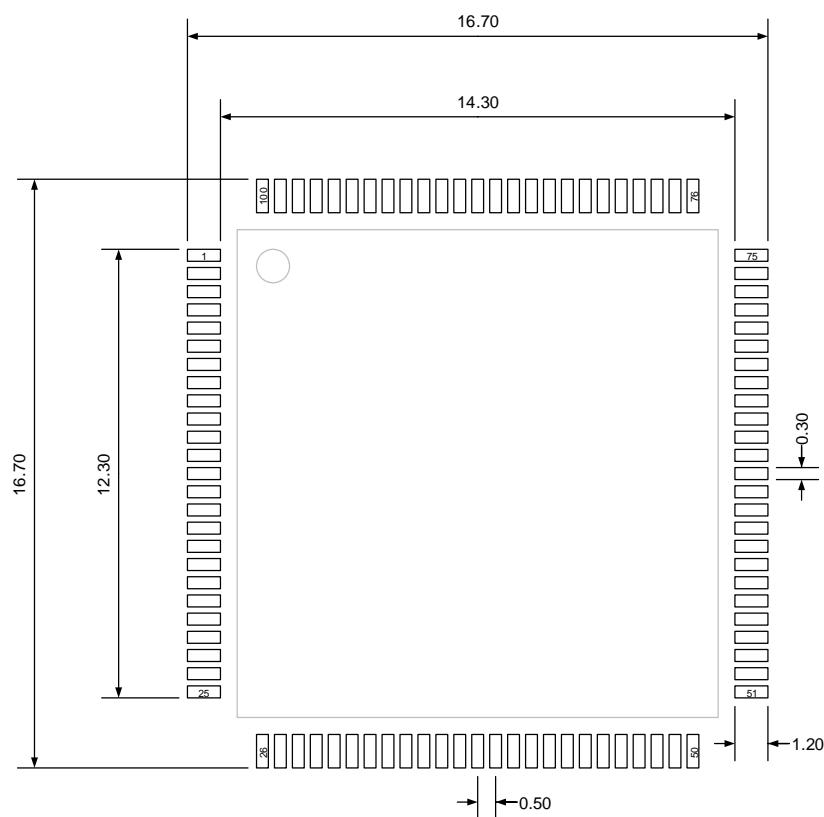
(Original dimensions are in millimeters)
