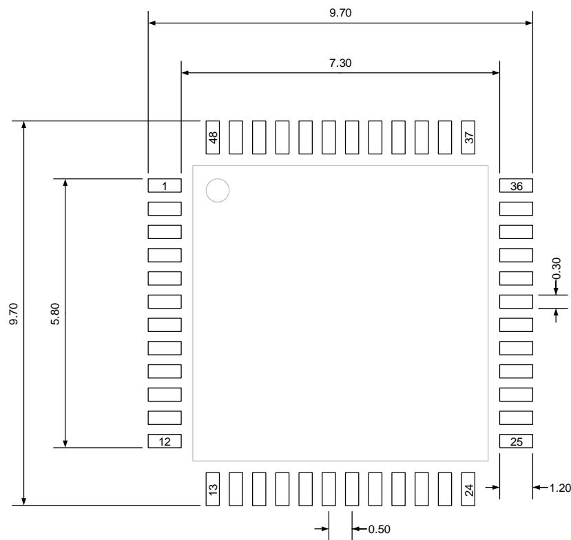
(Original dimensions are in millimeters)
