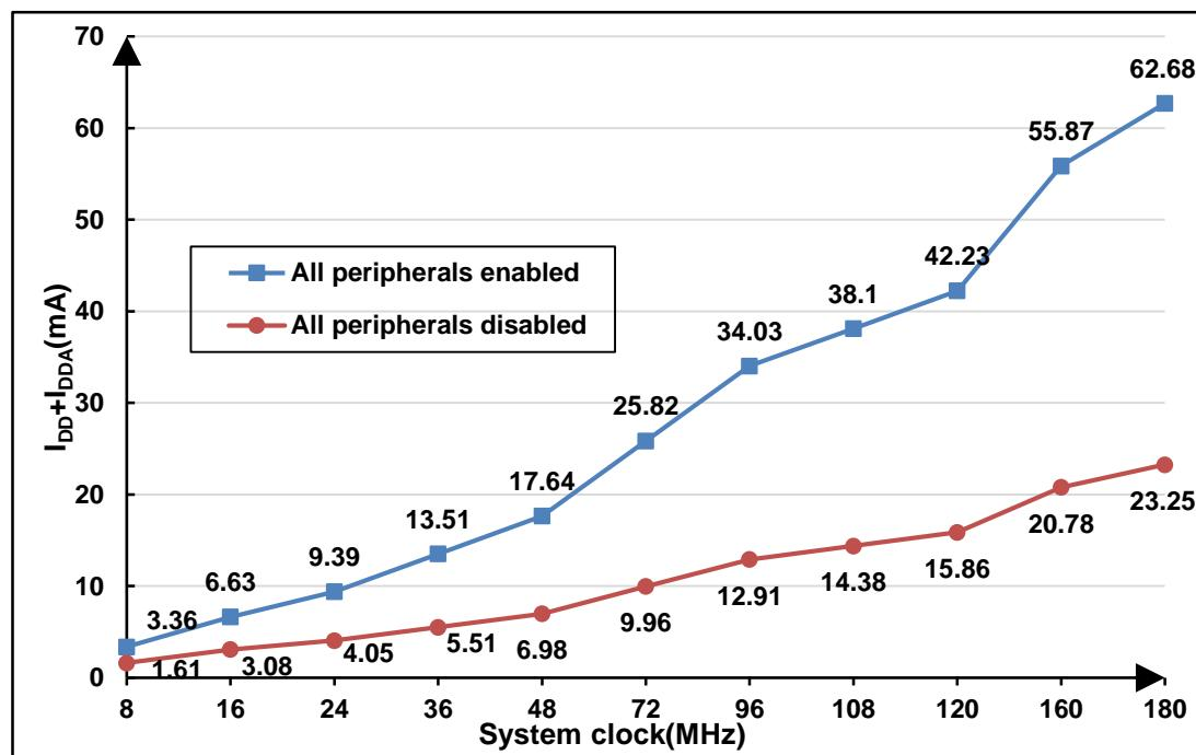
Figure 4-3. Typical supply current consumption in Sleep mode
