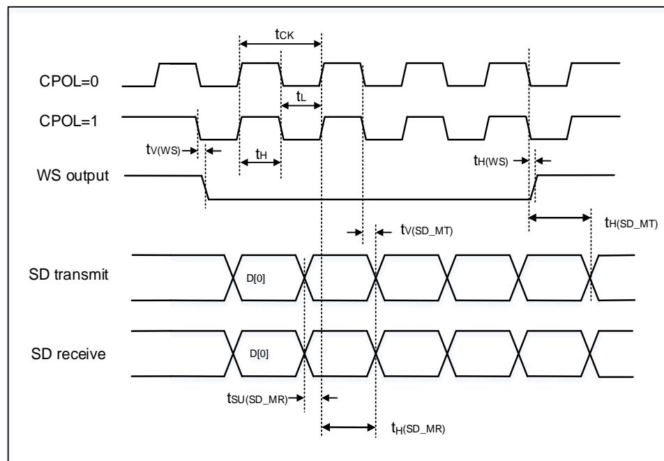
**Figure 4-10. I2S timing diagram - slave mode**
