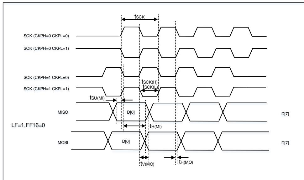
**Figure 4-8. SPI timing diagram - slave mode**
