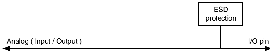
Figure 8-4. Basic structure of Analog configuration
