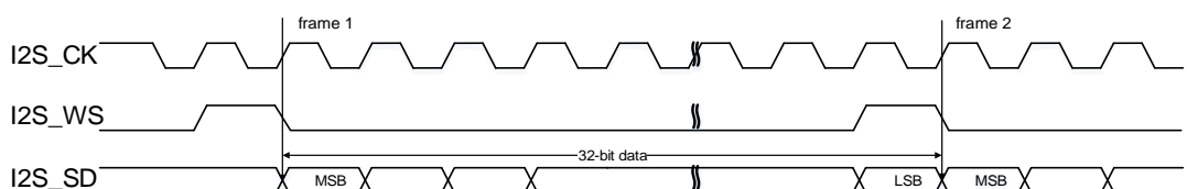
Figure 22-39. PCM standard short frame synchronization mode timing diagram (DTLEN=01, CHLEN=1, CKPL=0)
