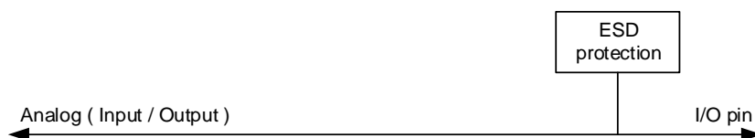
Figure 37-8. Basic structure of Analog configuration
