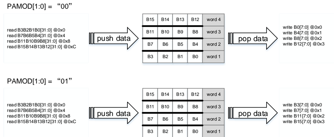
Figure 15-4. Data padding and alignment (source greater than destination)
