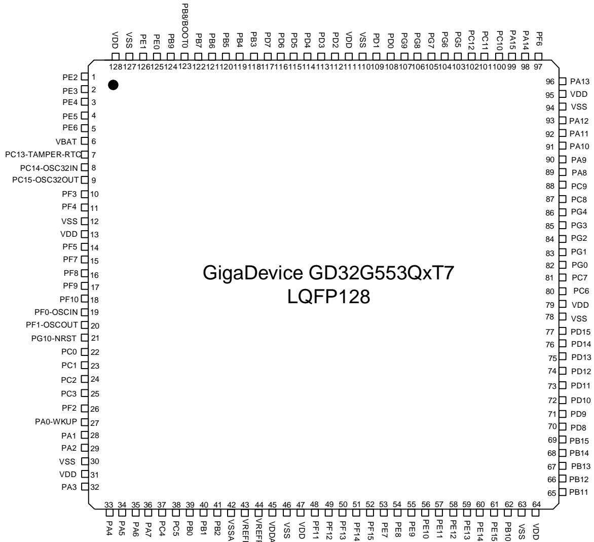
Figure 2-2. GD32G553QxT7 LQFP128 pinouts
