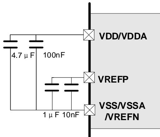
(1) All decoupling capacitors need to be as close as possible to the pins on the PCB board.
