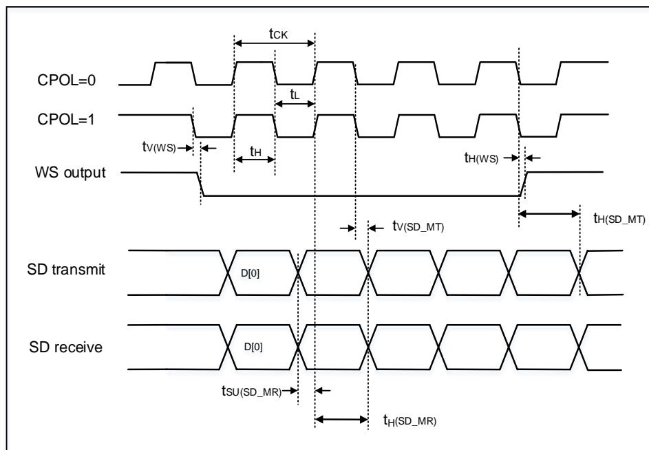
Figure 4-15. I2S timing diagram - slave mode
