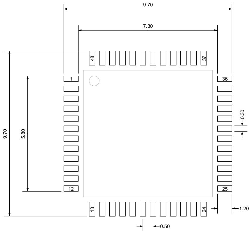
(Original dimensions are in millimeters)
