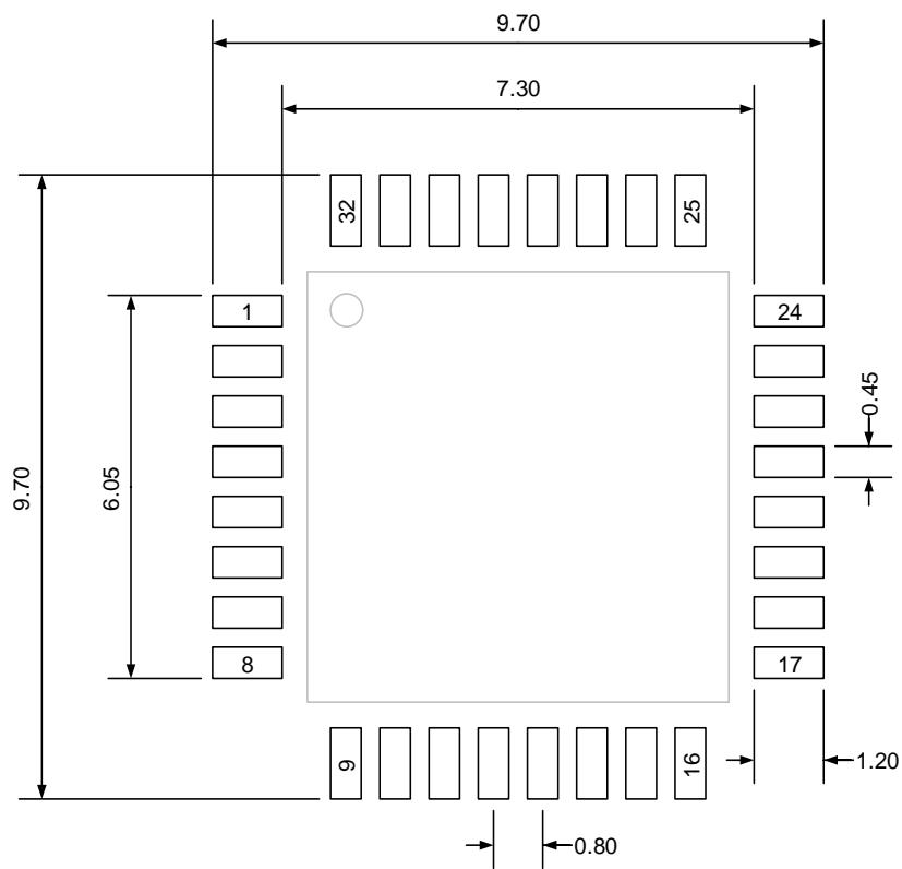
(Original dimensions are in millimeters)
