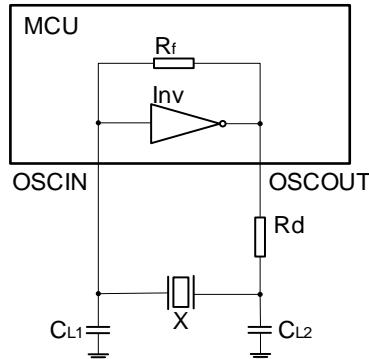
It is strongly recommended to measure the oscillation allowance (negative resistance) in the final target system (layout) to determine which load capacitors will best tune their resonator/crystal to the microcontroller device for optimum start-up and operation over temperature/voltage extremes.
