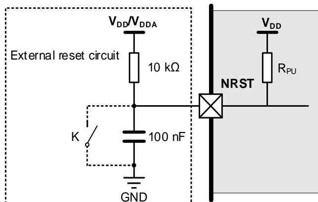
(1) Unless the voltage on NRST pin go below  $V_{IL(NRST)}$  level, the device would not generate a reliable reset.
