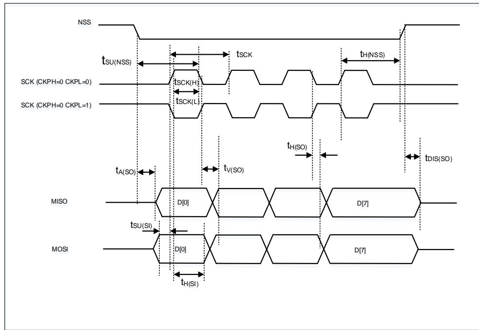
**Figure 4-13. SPI timing diagram - slave mode (CKPH=1)**
