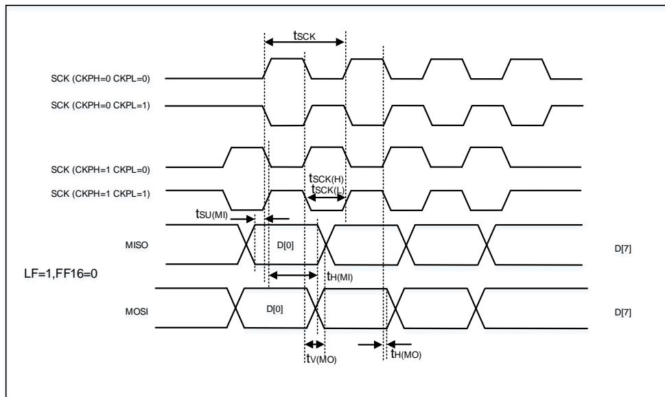
**Figure 4-12. SPI timing diagram - slave mode (CKPH=0)**
