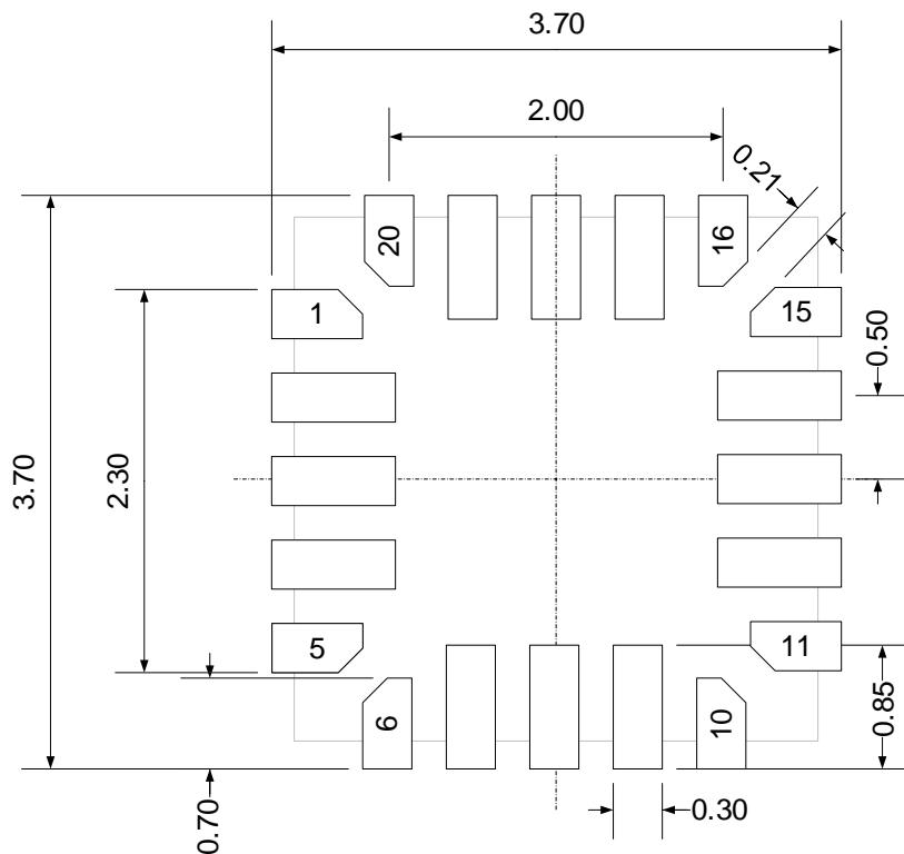
(Original dimensions are in millimeters)
