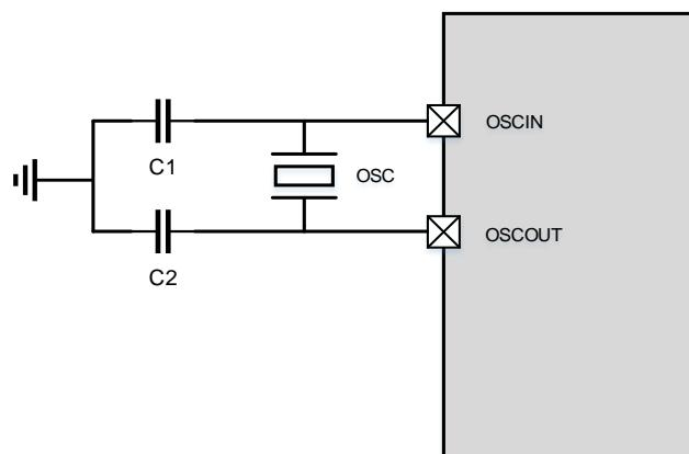
Figure 4-5. Recommended external OSCIN and OSCOUT pins circuit for oscillator
