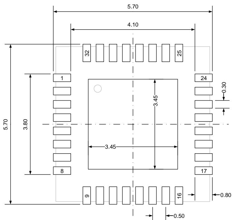
(Original dimensions are in millimeters)
